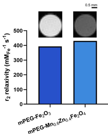
Fig. 5  $r_2$  relaxivity of mPEGylated  $\gamma$ -Fe<sub>2</sub>O<sub>3</sub> and Mn<sub>0.6</sub>Zn<sub>0.4</sub>Fe<sub>2</sub>O<sub>4</sub> measured at 9.4 T. The insets above the bars show the  $T_2$ -weighted images of the corresponding particles.
