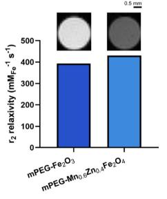
Fig. 5  $r_2$  relaxivity of mPEGylated  $\gamma$ -Fe<sub>2</sub>O<sub>3</sub> and Mn<sub>0.6</sub>Zn<sub>0.4</sub>Fe<sub>2</sub>O<sub>4</sub> measured at 9.4 T. The insets above the bars show the  $T_2$ -weighted images of the corresponding particles.
