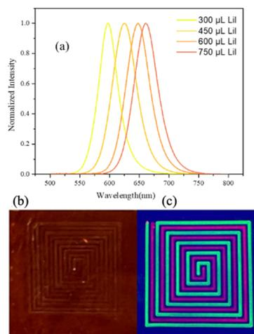
Fig. 5 (a) PL spectra of CsPbBr<sub>3</sub>-LiI nanocrystals with varying LiI concentrations. (b) Printed patterns observed under visible light. (c) Corresponding photoluminescent patterns under UV illumination.
