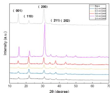
Fig. 1 XRD Patterns of CsPbBr<sub>3</sub> NCs modified with varying amounts of OAm.
