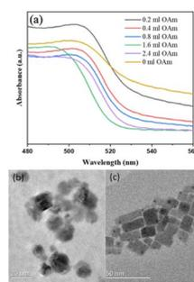
Fig. 3 (a) Normalized absorption spectra of CsPbBr<sub>3</sub> NCs synthesized with different volumes of OAm. (b) TEM image of CsPbBr<sub>3</sub> NCs without OAm. (c) TEM image of CsPbBr<sub>3</sub> with 1.6 mL OAm.
