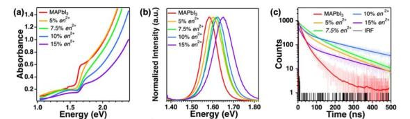
Fig. 2 (a) UV-Vis absorption spectra, (b) room-temperature steady-state PL spectra, and (c) time-resolved PL traces measured from {en}MAPbl<sub>3</sub> films with different en<sup>2+</sup> loadings. The solid lines in panel (c) represent the fitting results using a bi-exponential model convoluted with the instrument response function.
