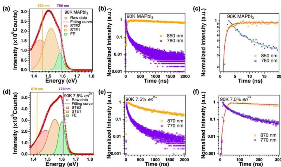
Fig. 7 Steady-state PL spectra of (a) pristine MAPbI<sub>3</sub> and (d) {en}MAPbI<sub>3</sub> with 7.5% en<sup>2+</sup> loading, measured at 90 K using 510 nm excitation. For each sample, the time-resolved PL traces were monitored at two wavelengths to track the dynamics of (b and c) FE and (e and f) STE emissions, respectively.
