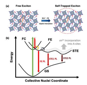
Fig. 6 (a) Illustrative diagram for the formation of a self-trapped exciton at low temperatures through the collective rearrangement of methylammonium cations in the orthorhombic phase of MAPbI<sub>3</sub>. (b) Potential energy diagram for the sequential evolution from the free carrier (FC) excited state to the free exciton (FE) state and, finally, to the self-trapped exciton (STE) state
