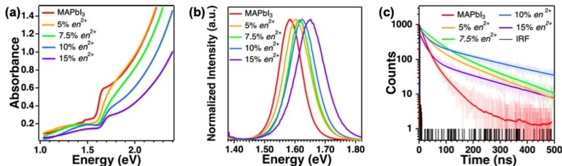
Fig. 2 (a) UV-Vis absorption spectra, (b) room-temperature steady-state PL spectra, and (c) time-resolved PL traces measured from  $\{en\}$ MAPbI<sub>3</sub> films with different  $en^{2+}$  loadings. The solid lines in panel (c) represent the fitting results using a bi-exponential model convoluted with the instrument response function.
