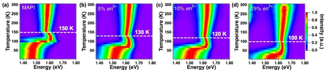
Fig. 3 Temperature-dependent PL spectra of (a) pristine MAPbI<sub>3</sub> and {en}MAPbI<sub>3</sub> films with (b) 5%, (c) 10%, and (d) 15% en<sup>2+</sup> loading. The tetragonal-to-orthorhombic phase transition temperatures are marked with dashed lines.
