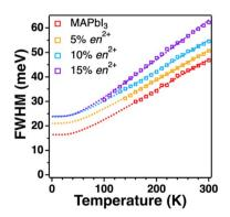
Fig. 4 The change of PL linewidths of  $\{en\}MAPbl_3$  films as a function of temperature. The dotted lines represent the fitting results obtained in the weak electron–phonon coupling limit, as described in the main text.
