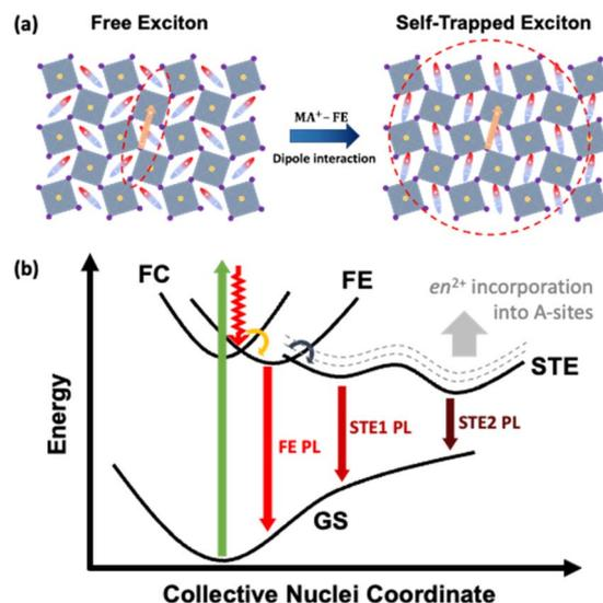
Fig. 6 (a) Illustrative diagram for the formation of a self-trapped exciton at low temperatures through the collective rearrangement of methylammonium cations in the orthorhombic phase of MAPbI<sub>3</sub>. (b) Potential energy diagram for the sequential evolution from the free carrier (FC) excited state to the free exciton (FE) state and, finally, to the self-trapped exciton (STE) state.
