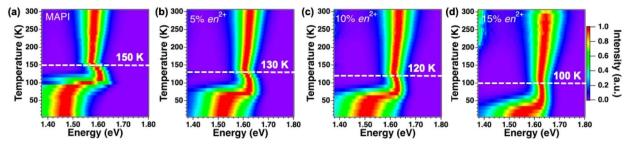
Fig. 3 Temperature-dependent PL spectra of (a) pristine MAPbI $_3$  and {en}MAPbI $_3$  films with (b) 5%, (c) 10%, and (d) 15% en $^{2+}$  loading. The tetragonal-to-orthorhombic phase transition temperatures are marked with dashed lines.
