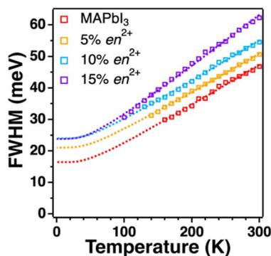
Fig. 4 The change of PL linewidths of {en}MAPbI<sub>3</sub> films as a function of temperature. The dotted lines represent the fitting results obtained in the weak electron-phonon coupling limit, as described in the main text.
