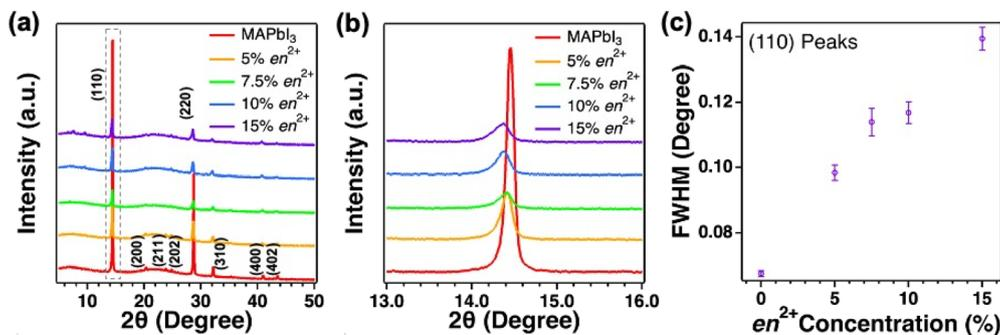
Fig. 1 (a) PXRD patterns of  $\{en\}$ MAPbI<sub>3</sub> films with different  $en^{2+}$  loadings. (b) Enlarged PXRD patterns around the MAPbI<sub>3</sub> (110) diffraction peak as enclosed by the grey dashed box in panel (a). (c) The change of the full width at half maxima of the tetragonal MAPbI<sub>3</sub> (110) reflection with  $en^{2+}$  loadings.
