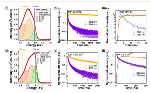
Fig. 7 Steady-state PL spectra of (a) pristine MAPbI<sub>3</sub> and (d)  $\{en\}MAPbI_3$  with 7.5%  $en^{2+}$  loading, measured at 90 K using 510 nm excitation. For each sample, the time-resolved PL traces were monitored at two wavelengths to track the dynamics of (b and c) FE and (e and f) STE emissions, respectively.
