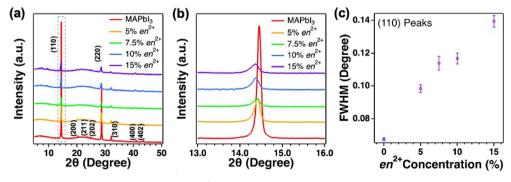
Fig. 1 (a) PXRD patterns of  $\{en\}$ MAPbl $_3$  films with different  $en^{2+}$  loadings. (b) Enlarged PXRD patterns around the MAPbl $_3$  (110) diffraction peak as enclosed by the grey dashed box in panel (a). (c) The change of the full width at half maxima of the tetragonal MAPbl $_3$  (110) reflection with  $en^{2+}$  loadings.
