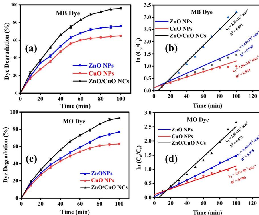
Fig. 6 Degradation efficiency versus time for (a) MB dye, (b) MO dye, (c) the reaction kinetics of MB dye (d) the reaction kinetics of MO dye. All results have been reported as mean  $\pm$  SD, with number of replicates ( $n$ ) = 3. Statistical significance was accepted at a level of  $p < 0.05$ .
