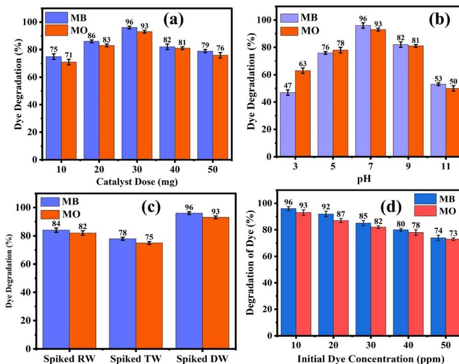
Fig. 7 Effect on dye degradation of various (a) catalyst doses, (b) pH values, (c) water matrixes, and (d) initial dye concentrations. All results have been reported as mean  $\pm$  SD, with number of replicates ( $n$ ) = 3. Statistical significance was accepted at a level of  $p < 0.05$ .
