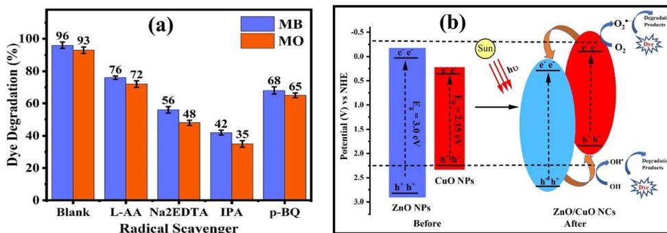
Fig. 8 (a) Effect of radical scavengers on dye degradation; (b) schematic illustration of band edge positions of  $E_{VB}$  and  $E_{CB}$  of ZnO NPs and CuO NPs, and proposed band alignment after the formation of a p-n heterojunction (ZnO/CuO NCs). All results have been reported as mean  $\pm$  SD, with number of replicates ( $n$ ) = 3. Statistical significance was accepted at a level of  $p < 0.05$ .
