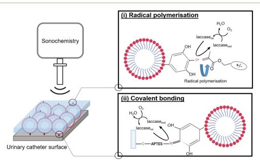
Fig. 3 Schematic representation of the bottom-up strategy for nano-enabled coating synthesis, illustrating the sono-enzymatic grafting of GaCeNPs and polymerisation of SB.
