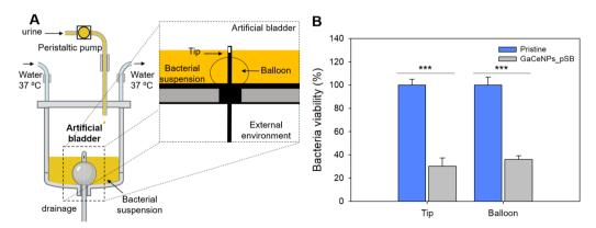
Fig. 8 (A) Schematic representation of the experimental setup simulating a human bladder. (B) Biofilm biomass quantification on pristine and GaCeNPs\_pSB-coated catheter sections (tip and balloon) following 7 days of incubation with recirculating infected urine in the artificial bladder system. Data are presented as the mean value  $\pm$  S.D. (n=3).
