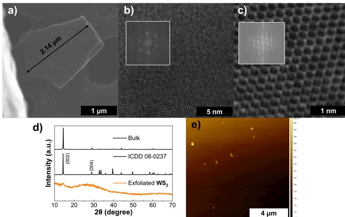
Fig. 7 Characterization of WS<sub>2</sub> ink: (a) HAADF-STEM of a large, exfoliated WS<sub>2</sub> sheet, (b) and (c) HAADF-STEM of a top-view of a nanosheet (the inset shows the power FFT patterns from the HAADF-STEM image) at different magnifications, (d) XRD spectra for WS<sub>2</sub> (bottom), reference WS<sub>2</sub> pattern ICDD 08-0237 (middle), and bulk MoS<sub>2</sub> flakes (top), (e) AFM scan of drop-casted ink diluted in IPA.
