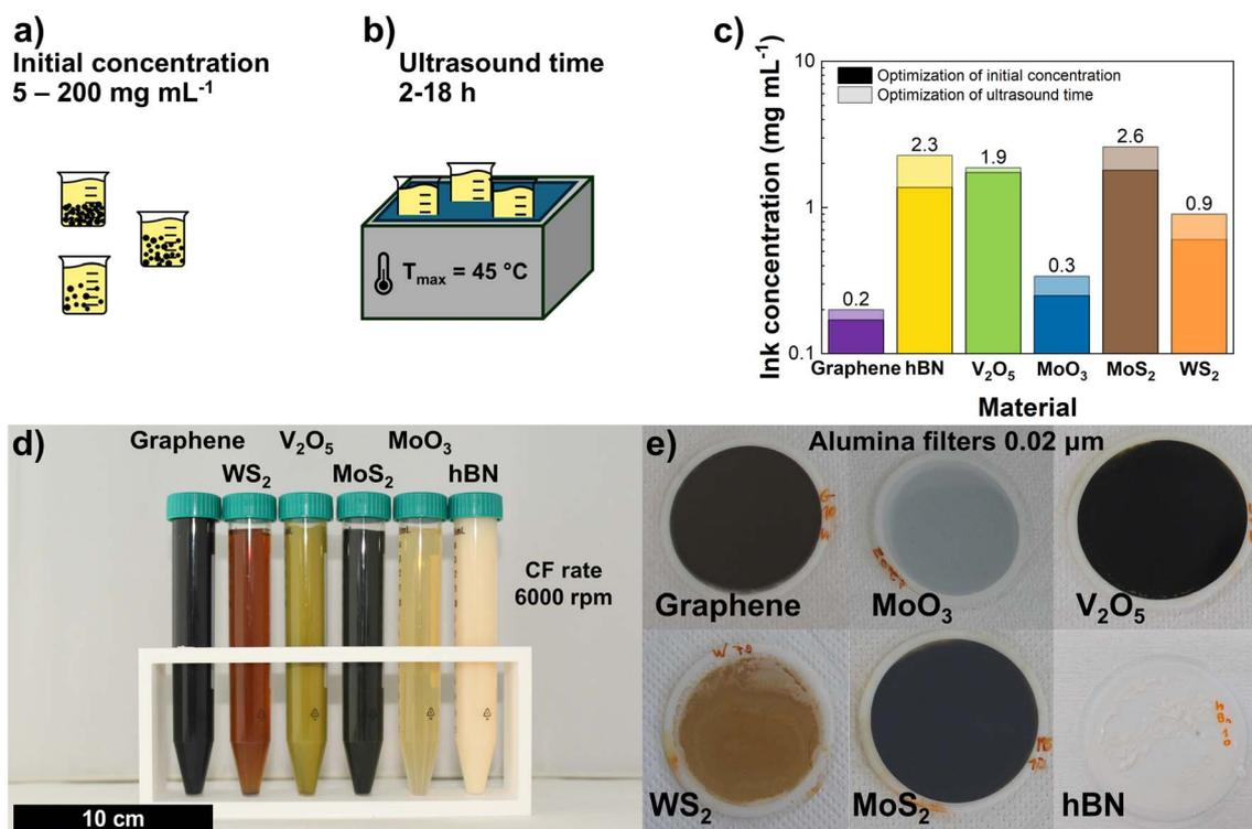
Fig. 1 Optimization of final concentration by varying: (a) initial concentration ( $5\text{--}200 \text{ mg mL}^{-1}$ ) and (b) ultrasound time ( $2\text{--}18 \text{ h}$ ). (c) Highest concentrations obtained in each series for all materials. (d) Optimized inks and (e) filtered inks in  $0.02 \mu\text{m}$  alumina filters.
