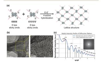
Fig. 5 (a) Schematic illustration of the 6 bps-DNA conjugated isotetravalent DTHBs and the assembly of lattice structures. (b) TEM images of the resulting lattice structures. (c) Radial intensity profile obtained from selected area electron diffraction (SAED) of the lattice shown in (b), overlaid with the theoretical diffraction pattern for diamond cubic lattice. The inset shows the corresponding diffraction image.
