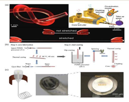
Fig. 6 Stretchable optical strain sensors are being manufactured. (a) The optical waveguides made of stretchable thermoplastic elastomer undergo coextrusion. (b) Stretchable optical fibers are made in two steps using a core/cladding step-index structure. (c) Using heat drawing to create superelastic multimaterial optical fibers. Reproduced from ref. 106. With permission from [WILEY], copyright [2019].
