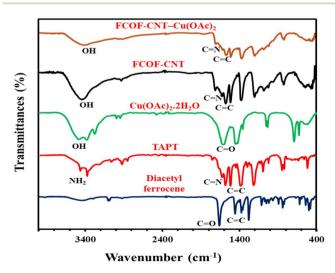
Fig. 1 FT-IR spectra of FCOF-CNT-Cu(OAc)<sub>2</sub> and its intermediates.
