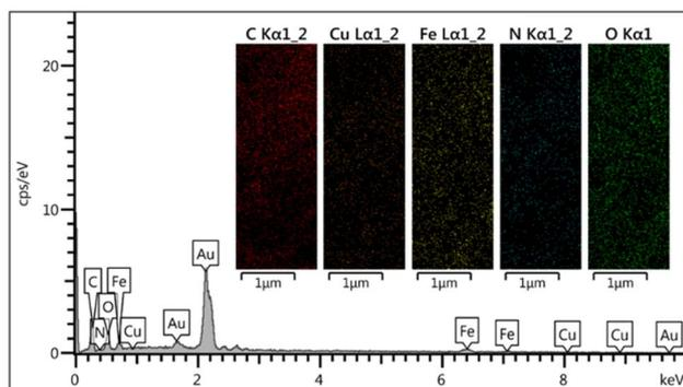
Fig. 8 EDS signals and mapping images of recovered COF-CNT-Cu(OAc)<sub>2</sub>.
