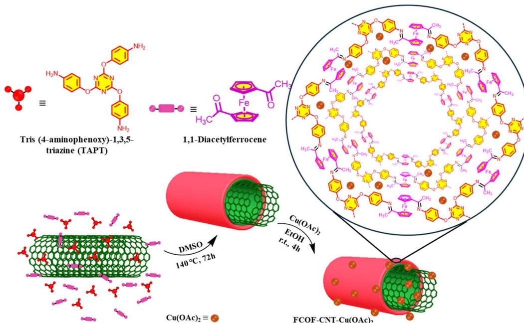
Scheme 1 Schematic of the fabrication of FCOF-CNT-Cu(OAc)<sub>2</sub>.
