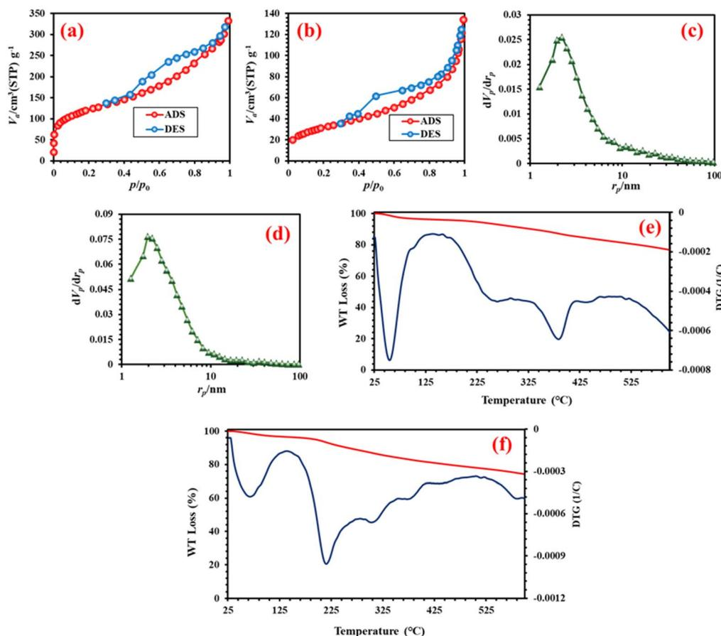
Fig. 6 N<sub>2</sub> adsorption/desorption isotherms of FCOF-CNT (a) and FCOF-CNT-Cu(OAc)<sub>2</sub>. (b) Pore size distribution of FCOF-CNT (c) and FCOF-CNT-Cu(OAc)<sub>2</sub>. (d) TGA/DTG curves of FCOF-CNT and (e) FCOF-CNT-Cu(OAc)<sub>2</sub> (f).
