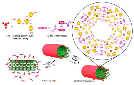
Scheme 1 Schematic of the fabrication of FCOF-CNT-Cu(OAc)<sub>2</sub>.
