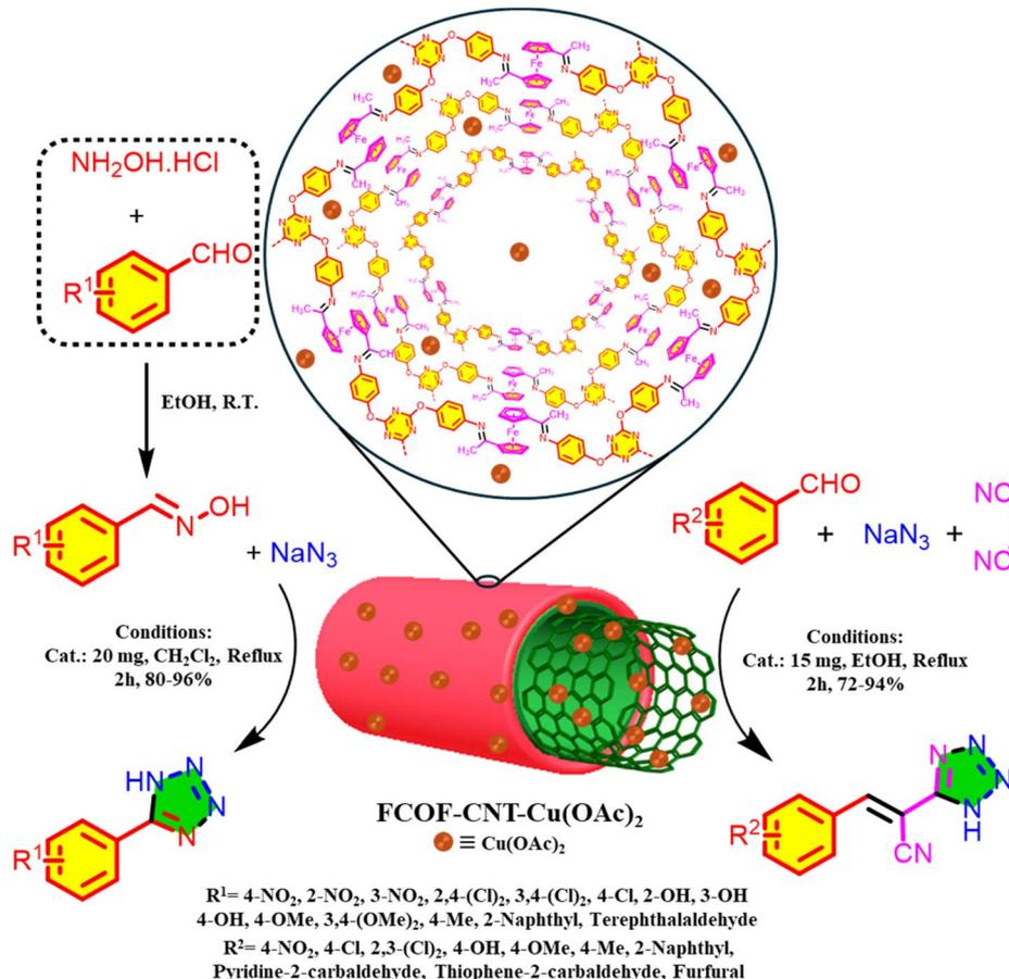
Scheme 2 Catalytic preparation of tetrazole derivatives using FCOF-CNT-Cu(OAc)<sub>2</sub>.
