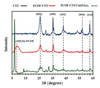
Fig. 2 XRD patterns of CNT, FCOF-CNT and FCOF-CNT-Cu(OAc)<sub>2</sub>.
