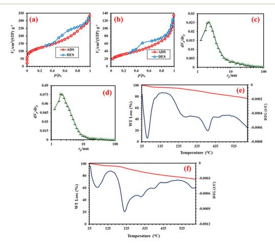
Fig. 6  $N_2$  adsorption/desorption isotherms of FCOF-CNT (a) and FCOF-CNT-Cu(OAc)<sub>2</sub>. (b) Pore size distribution of FCOF-CNT (c) and FCOF-CNT-Cu(OAc)<sub>2</sub>. (d) TGA/DTG curves of FCOF-CNT and (e) FCOF-CNT-Cu(OAc)<sub>2</sub> (f).
