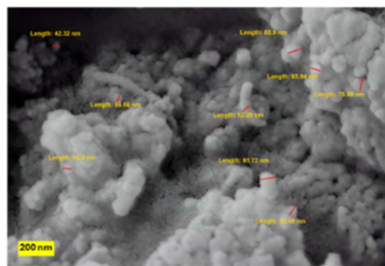
Fig. 7 FE-SEM image of recovered FCOF-CNT-Cu(OAc) 2 .
