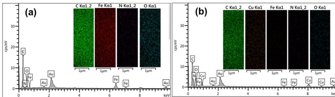
Fig. 5 EDS mapping results of FCOF-CNT (a) and FCOF-CNT-Cu(OAc)<sub>2</sub> (b).
