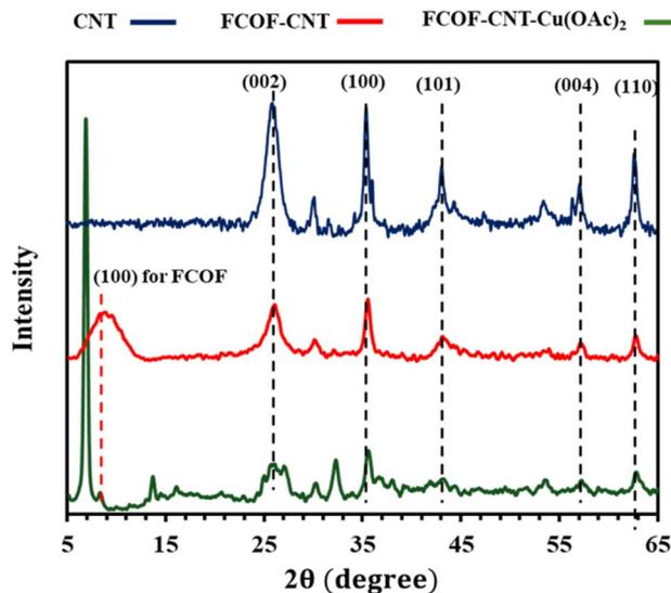
Fig. 2 XRD patterns of CNT, FCOF-CNT and FCOF-CNT-Cu(OAc)<sub>2</sub>.
