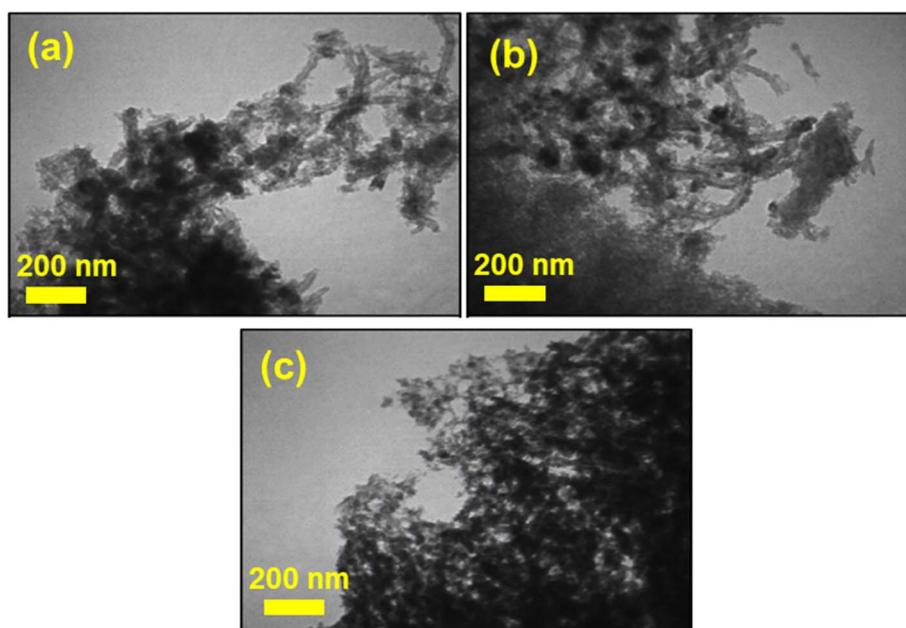
Fig. 4 TEM images of FCOF-CNT (a, b) and FCOF-CNT-Cu(OAc)<sub>2</sub> (c).
