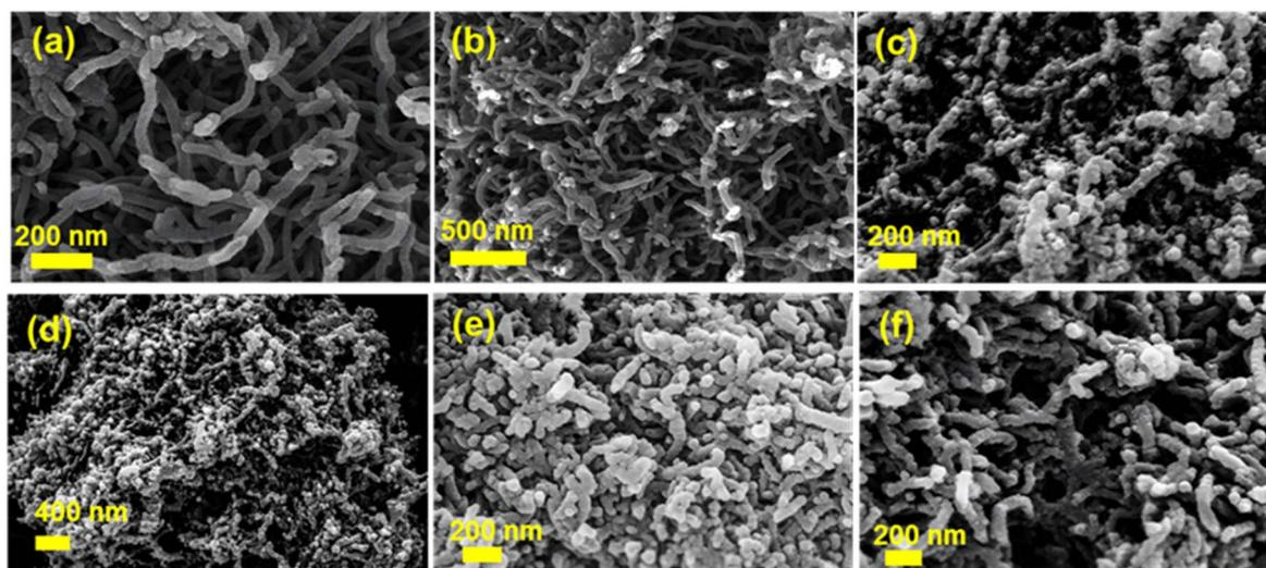
Fig. 3 FE-SEM images of CNT (a, b), FCOF-CNT (c, d) and FCOF-CNT-Cu(OAc)<sub>2</sub> (e, f).
