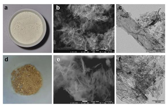
Fig. 2 Characterization of  $CeO_2$  and  $Rf-CeO_2$  NPs. (a)  $CeO_2$  and (d)  $Rf-CeO_2$ . Field-emission scanning electron microscopy images of  $CeO_2$  (b) and  $Rf-CeO_2$  (e). Transmission electron microscopy images of  $CeO_2$  (c) and  $Rf-CeO_2$  (f). Both NPs exhibit a well-defined, rod-shaped morphology with an average particle size of < 50 nm.
