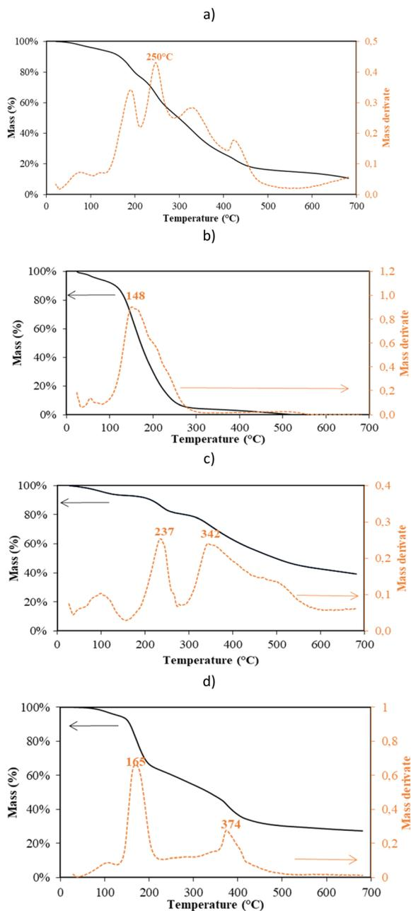
Fig. 7 Thermogravimetric curves for (a) CQD-diethanolamine, (b) CQD-diethylamine, (c) CQD-ethylenediamine, and (d) CQD-phenylenediamine, using a heating ramp of  $20\text{ }^{\circ}\text{C min}^{-1}$  from  $50\text{ }^{\circ}\text{C}$  to  $800\text{ }^{\circ}\text{C}$  under an air flow of  $80\text{ mL min}^{-1}$ .
