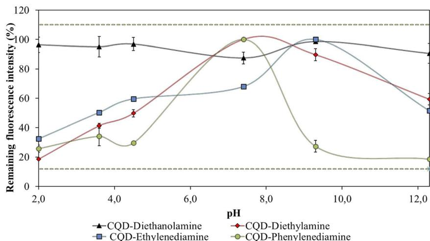
Fig. 15 Effect of pH on the fluorescence of CQD-diethanolamine, CQD-diethylamine, CQD-ethylenediamine, and CQD-phenylenediamine prepared by dispersion in water at  $100 \text{ mg L}^{-1}$ .
