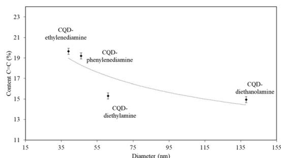
Fig. 8 Correlation between the content of  $\text{C}=\text{C}$  and the hydrodynamic diameter of the synthesized CQDs.
