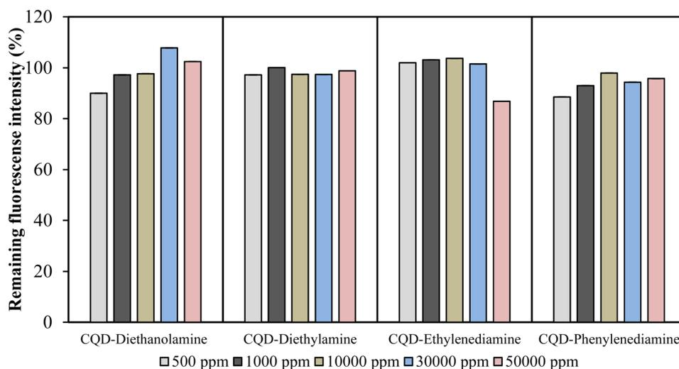
Fig. 13 Effect of ionic strength on the fluorescence of the N-CQDs prepared by dispersion in brine of the NaCl at 500, 1000, 10 000, 30 000, and 50 000 mg L<sup>-1</sup>.
