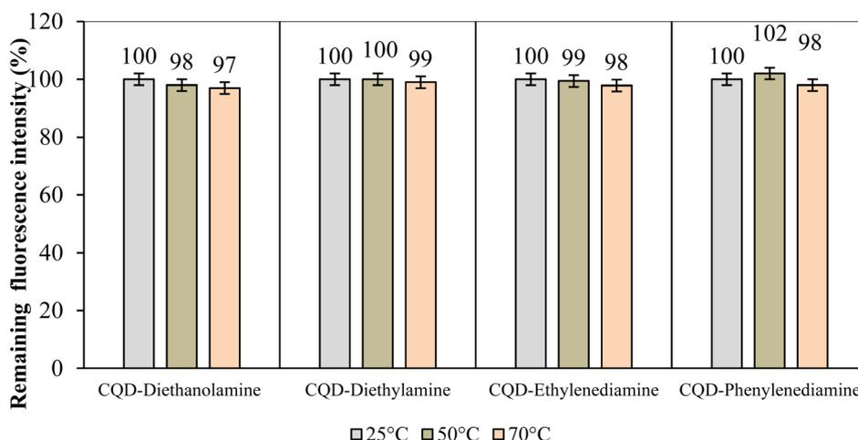
Fig. 12 Thermal stability evaluated through changes in the fluorescence for the N-CQDs prepared by dispersion in distilled water at 100 mg L<sup>-1</sup> and subjected to 25, 50 and 70 °C.
