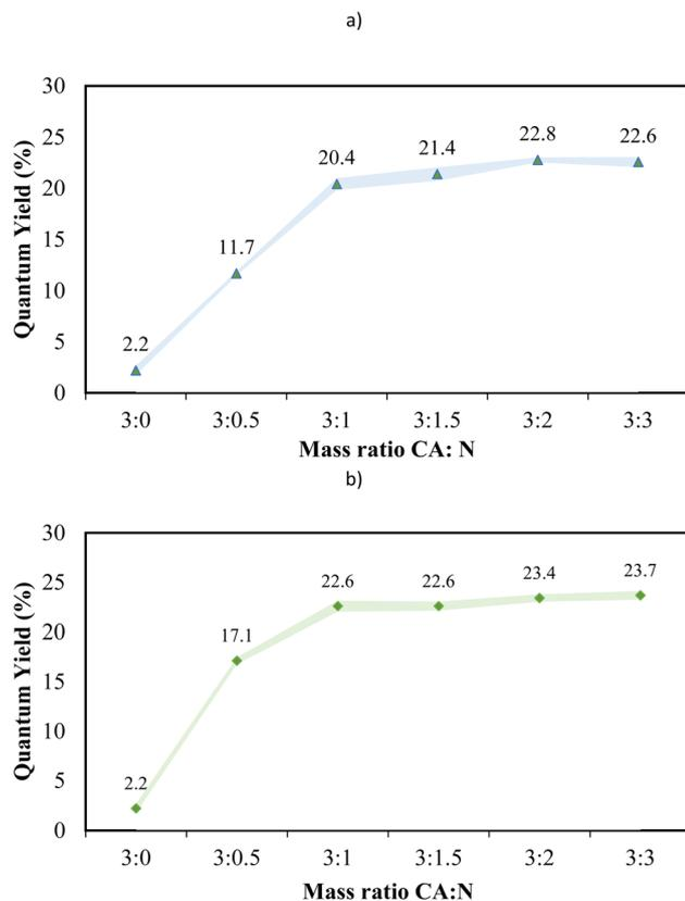
Fig. 11 The QY dependence on citric acid : N-precursor mass ratio used during the synthesis of (a) CQD-ethylenediamine and (b) CQD-phenylenediamine.
