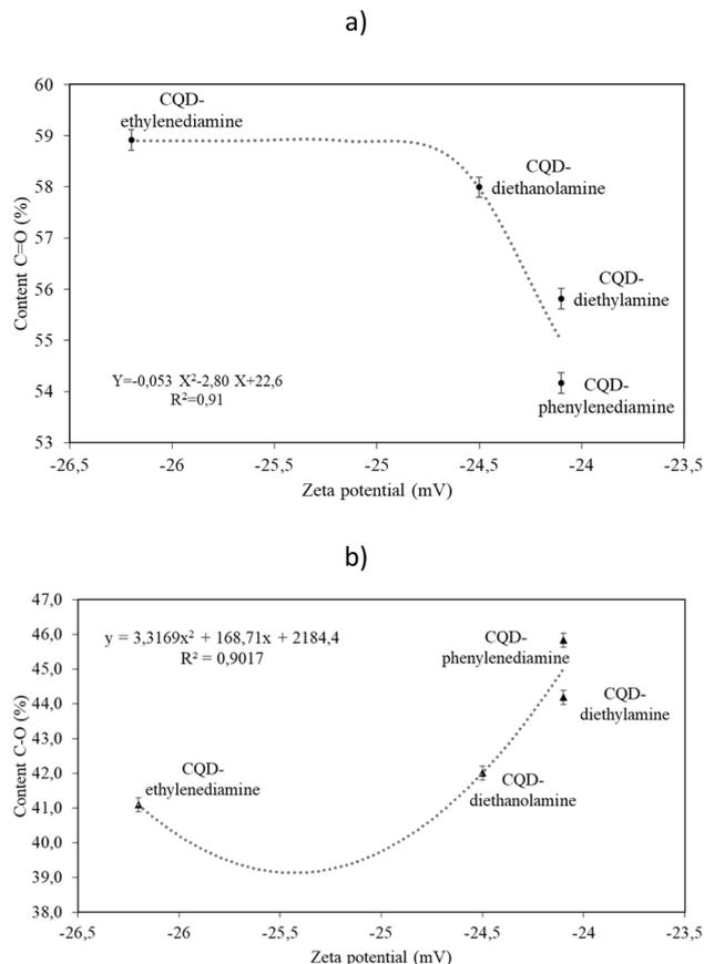
Fig. 4 Correlation between the z-potential and (a) the percentage of  $C=O$  content present on the surface of the synthesized CQDs and (b) the percentage of  $C-O$  content present on the surface of the synthesized CQDs.
