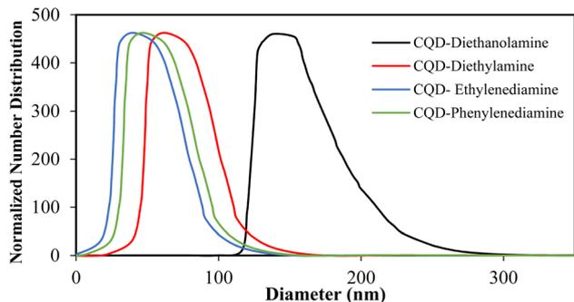
Fig. 5 Hydrodynamic diameter by DLS for synthesized N-CQDs.
