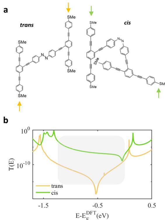
Fig. 4 (a) Schematic illustration of the two OPE3-based structures with *E* and *Z* conformations. (b) Transmission coefficient  $T(E)$  of both junctions against electron energy  $E$ , obtained when electrodes are connected to the SMe groups indicated by arrows.
