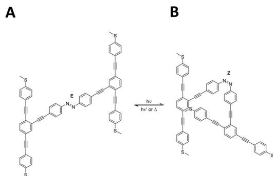
**Fig. 2** Schematic illustration of the OPE3-based molecule in an *E* or *Z* isomer under light stimulus, labelled A and B, respectively. A total energy difference of 0.04 eV is calculated between the fully relaxed geometries of the two isomers.
