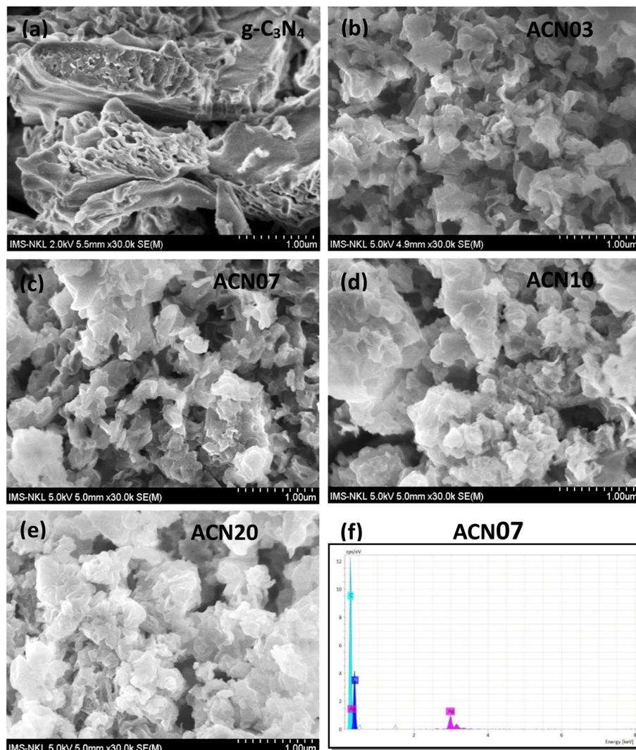
Fig. 2 FESEM images of the ACN nanocomposite samples: (a) g-C<sub>3</sub>N<sub>4</sub>, (b) ACN03, (c) ACN07, (d) ACN10, and (e) ACN20. (f) EDX spectrum of the ACN07 sample.
