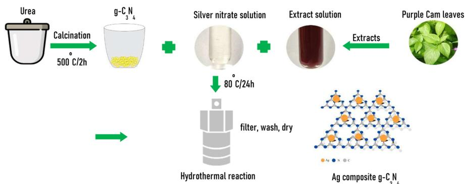
Scheme 1 Schematic of the preparation process of  $\text{Ag}@g\text{-C}_3\text{N}_4$  nanocomposites.
