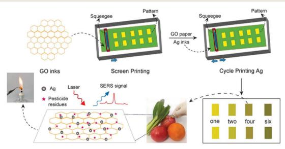
Fig. 9 Scheme illustrating the fabrication process of the SERS paper by screen-printing and its use as a swab to quantify thiram, thiabendazole, and methyl parathion in fruits and vegetables. This figure has been adapted/reproduced from ref. 103 with permission from Royal Society of Chemistry, copyright 2025
