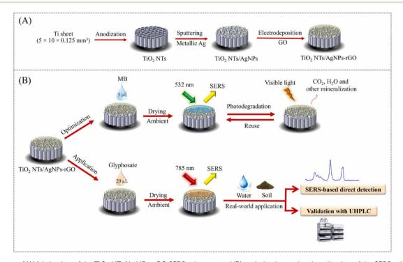
Fig. 8 Scheme of (A) fabrication of the TiO<sub>2</sub> NTs/AqNPs-rGO SERS substrate and (B) optimization and real application of the SERS substrate. This figure has been adapted/reproduced from ref. 151 with permission from Elsevier, copyright 2025.
