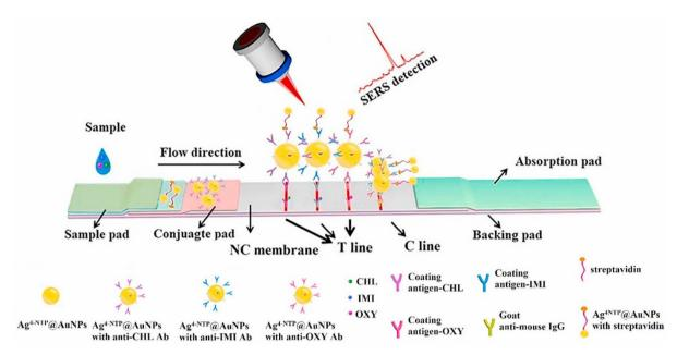
Fig. 12 Scheme of the LFA-SERS strategy using enhanced Ag<sup>4-NTP</sup>@Au for the multiplex strip. This figure has been adapted/reproduced from ref. 189 with permission from Elsevier, copyright 2025.
