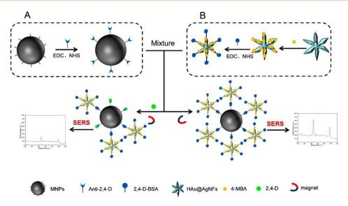
Fig. 10 Schematic illustration of the strategy used for 2,4-D analysis using an Au@Ag@MBA-antigen SERS-tag. (A) Functionalization of magnetic nanoparticles (MNPs) with anti-2,4-D for selective recognition. (B) Preparation of Au@Ag nanoflowers labeled with 4-MBA and conjugated with 2,4-D-BSA. This figure has been adapted/reproduced from ref. 104 with permission from Elsevier, copyright 2025
