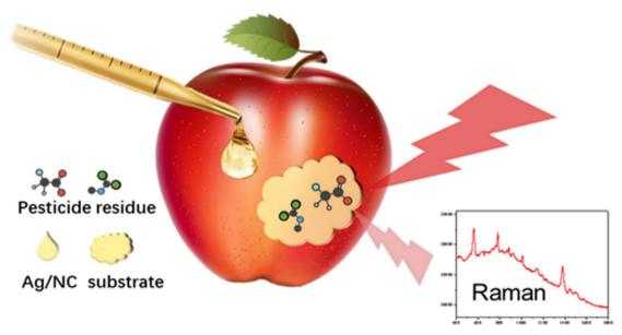
Fig. 5 Scheme for SERS analysis of thiram and thiabendazole in apple peels using AgNP@NC as the substrate. This figure has been adapted/ reproduced from ref. 112 with permission from Elsevier, copyright 2025.
