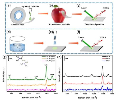
Fig. 7 Scheme illustrating (a) – (c) the procedure of preparing a flexible SERS substrate for extracting and detecting pesticides on apple surfaces. (d)-(f) Schematic showing the SERS detection of pesticides in river water. (g) SERS spectra of thiram with different concentrations extracted from the apple surface. (h) SERS spectra of thiram in river water. This figure has been adapted/reproduced from ref. 123 with permission from Springer Nature, copyright 2025.
