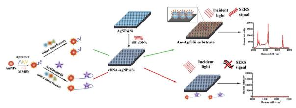
Fig. 11 Schematic of SERS aptasensor substrate fabrication and mechanism for acetamiprid detection. This figure has been adapted/reproduced from ref. 178 with permission from Elsevier, copyright 2025.
