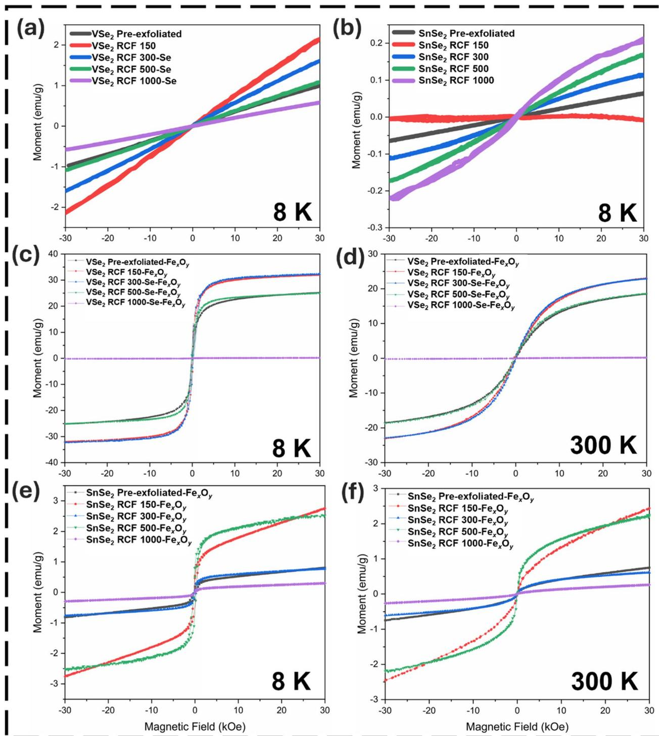
Fig. 4 Magnetization curves for various samples. (a) VSe<sub>2</sub> and (b) SnSe<sub>2</sub> measured at 8 K. VSe<sub>2</sub> decorated with Fe<sub>x</sub>O<sub>y</sub> measured at (c) 8 K and (d) 300 K. SnSe<sub>2</sub> decorated with Fe<sub>x</sub>O<sub>y</sub> measured at (e) 8 K and (f) 300 K.
