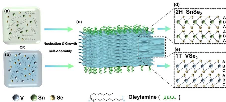
**Scheme 1** Solution-phase synthesis of 2D layered nanosheets. (a) VO(acac)<sub>2</sub> or (b) Sn(acac)<sub>2</sub>, along with Se, was dissolved separately in oleylamine, where each reacted individually (in separate experiments) to form (c) bulk nanostructured materials, resulting in (d) 2H-SnSe<sub>2</sub> or (e) 1T-VSe<sub>2</sub> nanostructures, respectively.
