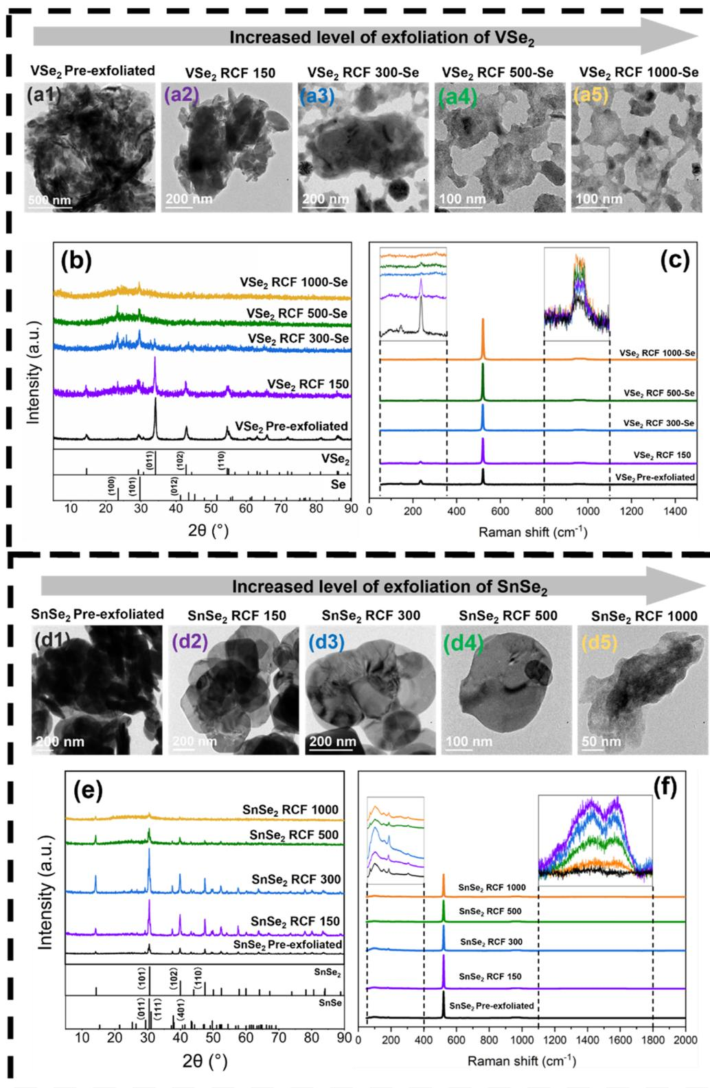
Fig. 2 Characterization of  $\text{VSe}_2$  and  $\text{SnSe}_2$  nanosheets. (a) Panels (a1)–(a5) show representative TEM images for different levels of exfoliation of  $\text{VSe}_2$ ; (b) XRD patterns and (c) Raman spectra for the  $\text{VSe}_2$  samples as labeled. (d) Panels (d1)–(d5) provide representative TEM images for different levels of exfoliation of  $\text{SnSe}_2$ ; (e) XRD patterns and (f) Raman spectra for  $\text{SnSe}_2$  samples as labeled.
