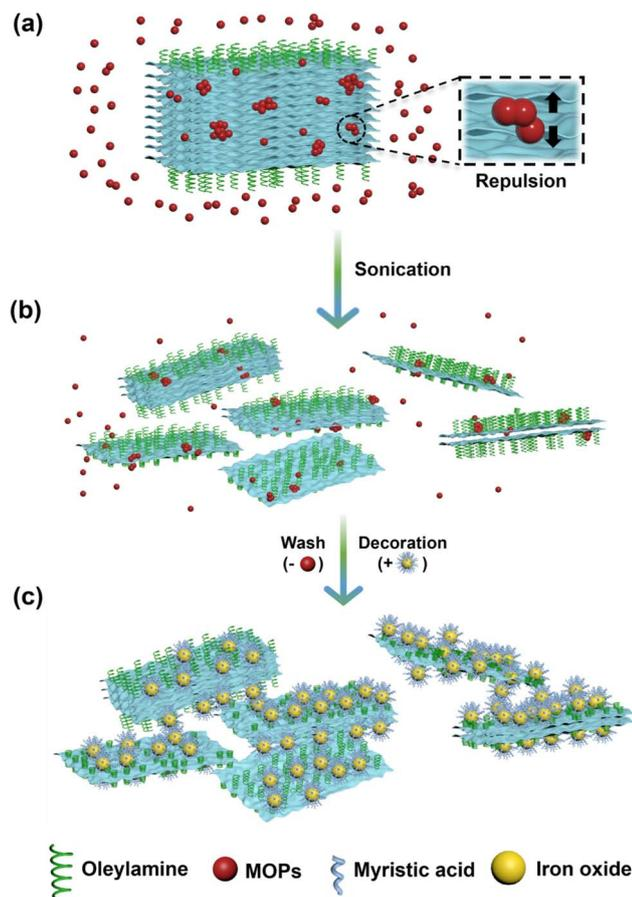
**Fig. 1** Mechanism of redox exfoliation of TMDs and their decoration with  $\text{Fe}_x\text{O}_y$ . (a) MOPs (red) assemble into polyoxometalates and adsorb on the bulk material during reduction. (b) Bulk materials are exfoliated to layered nanostructures of varying thickness. (c)  $\text{Fe}_x\text{O}_y$  (yellow) with myristic acid (blue) on their surfaces are coupled with exfoliated nanosheets.
