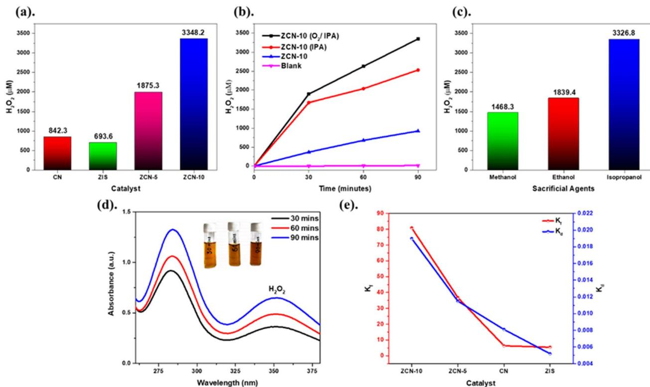
Fig. 7 (a) Effect of various catalysts, (b) effect of  $O_2$  purging, (c) effect of sacrificial agents, (d) absorbance peaks for  $H_2O_2$  concentration with time, and (e) kinetics study for photocatalytic  $H_2O_2$  production.
