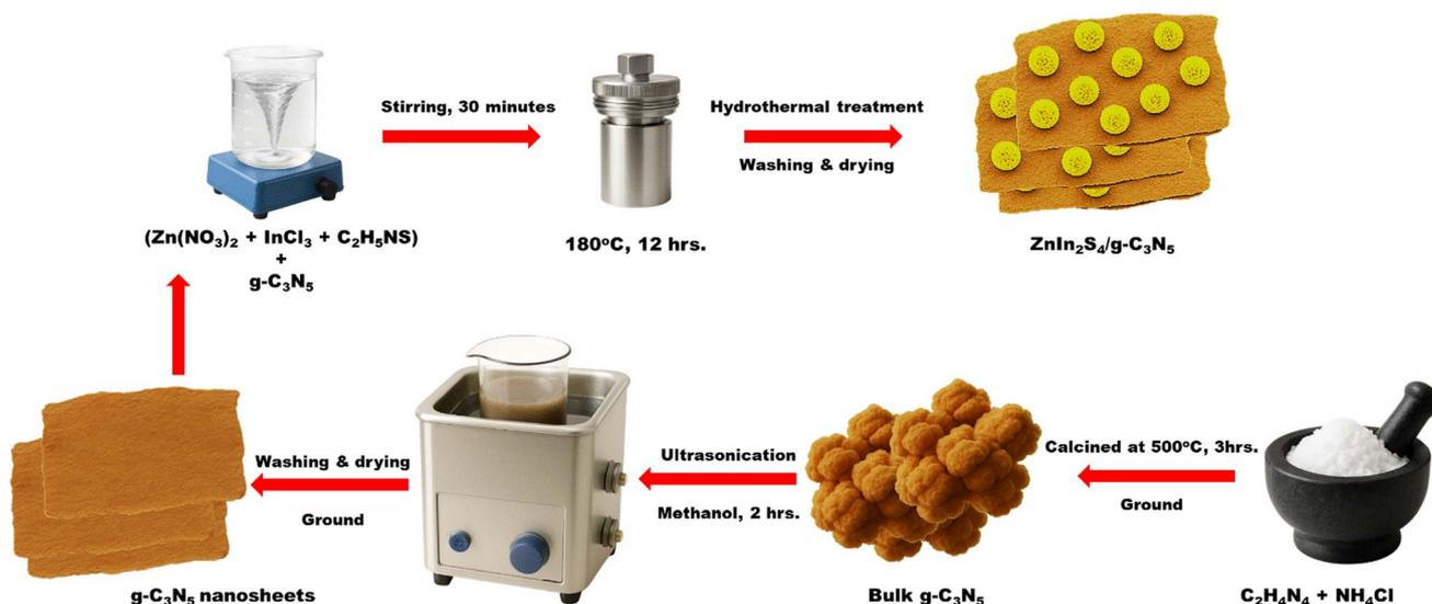
Scheme 1 Schematic illustration for synthesis of ZnIn<sub>2</sub>S<sub>4</sub>, g-C<sub>3</sub>N<sub>5</sub> and ZnIn<sub>2</sub>S<sub>4</sub>/g-C<sub>3</sub>N<sub>5</sub> composites.
