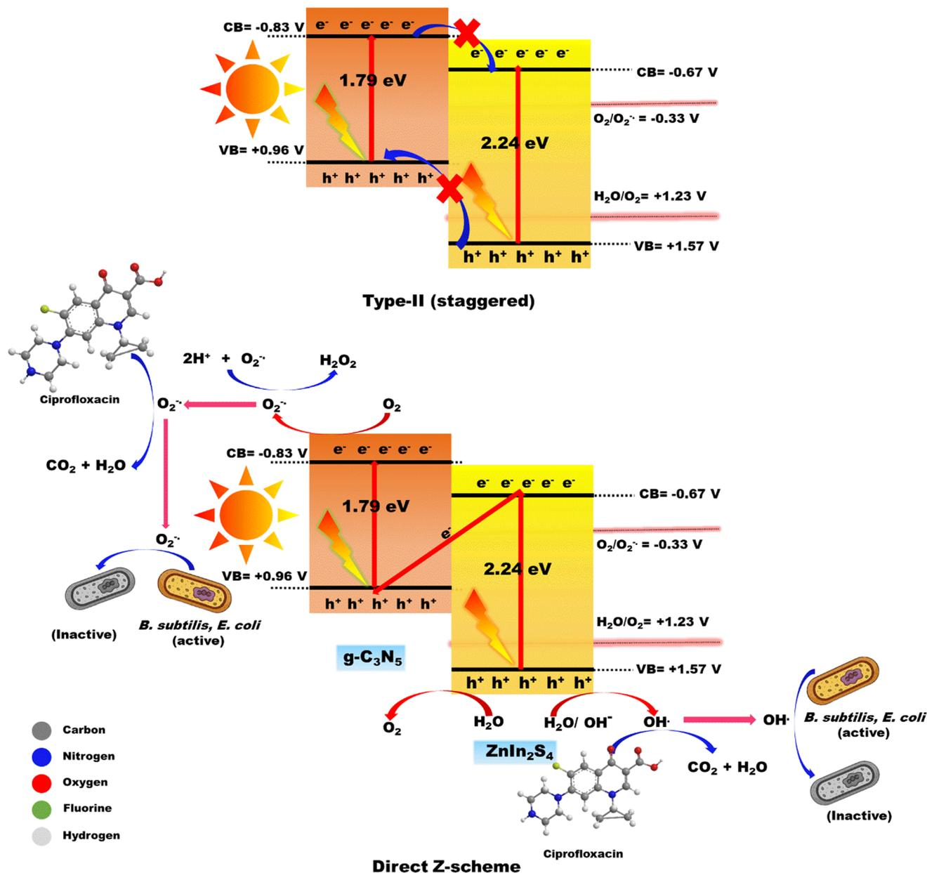
Scheme 2 Plausible mechanism for photocatalytic CIP degradation, H<sub>2</sub>O<sub>2</sub> production, and antimicrobial activity against *B. subtilis* for the ZCN-10 composite.
