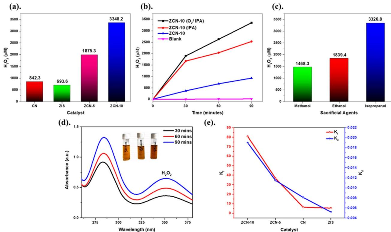
Fig. 7 (a) Effect of various catalysts, (b) effect of O<sub>2</sub> purging, (c) effect of sacrificial agents, (d) absorbance peaks for H<sub>2</sub>O<sub>2</sub> concentration with time, and (e) kinetics study for photocatalytic H<sub>2</sub>O<sub>2</sub> production.
