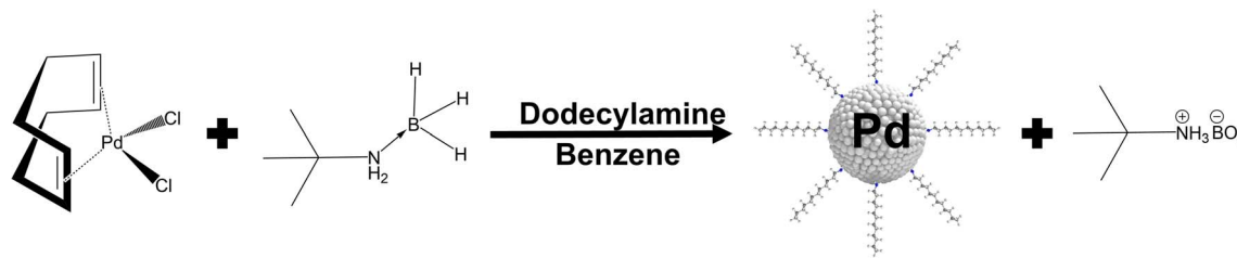
Fig. 1 Synthesis of ultrasmall palladium nanoparticles. Dichlorido(1,5-cyclooctadiene)palladium(II) is reduced with tert -butylamine borane in benzene and stabilized by the capping ligand n -dodecylamine.
