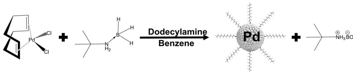
Fig. 1 Synthesis of ultrasmall palladium nanoparticles. Dichlorido(1,5-cyclooctadiene)palladium(II) is reduced with *tert*-butylamine borane in benzene and stabilized by the capping ligand *n*-dodecylamine.
