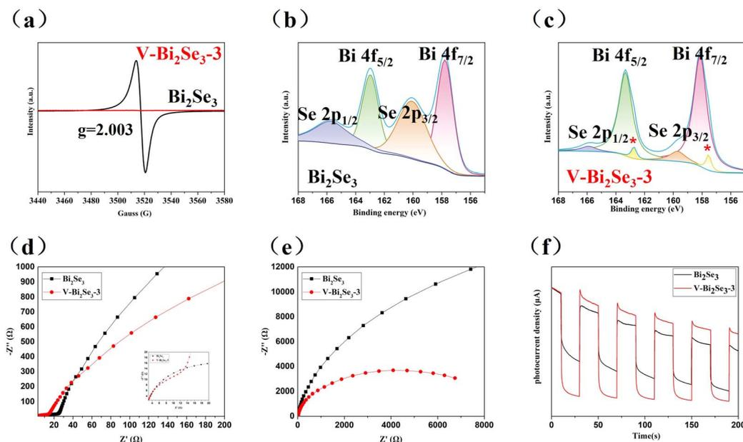
Fig. 2 (a) EPR spectra of  $\text{Bi}_2\text{Se}_3$  and  $\text{V-Bi}_2\text{Se}_3\text{-3}$ ; (b) XPS spectra of  $\text{Bi}_2\text{Se}_3$  for Bi 4f and Se 2p; (c) XPS spectra of  $\text{V-Bi}_2\text{Se}_3\text{-3}$  for Bi 4f and Se 2p; (d and e) impedance spectra of  $\text{Bi}_2\text{Se}_3$  and  $\text{V-Bi}_2\text{Se}_3\text{-3}$  in high, medium and low frequency regions; (f) photocurrent spectra of  $\text{V-Bi}_2\text{Se}_3\text{-3}$ .
