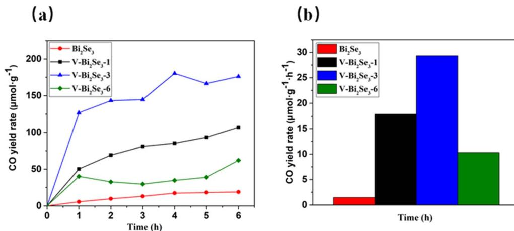
Fig. 3 (a) Photocatalytic CO evolution under 300 W Xe lamp irradiation for 6 h with different samples. (b) Comparison of the photocatalytic CO<sub>2</sub> reduction activity with different samples.
