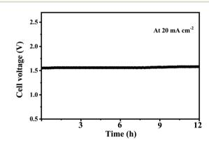
Fig. 8 Overall water splitting performance of NCMCSP during a 12 h chronopotentiometry test.
