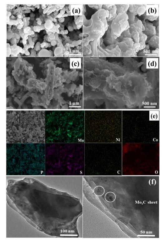
Fig. 4 FESEM images of NCMC (a and b) and NCMCSP (c and d). Elemental mapping of NCMCSP (e). TEM images (f).
