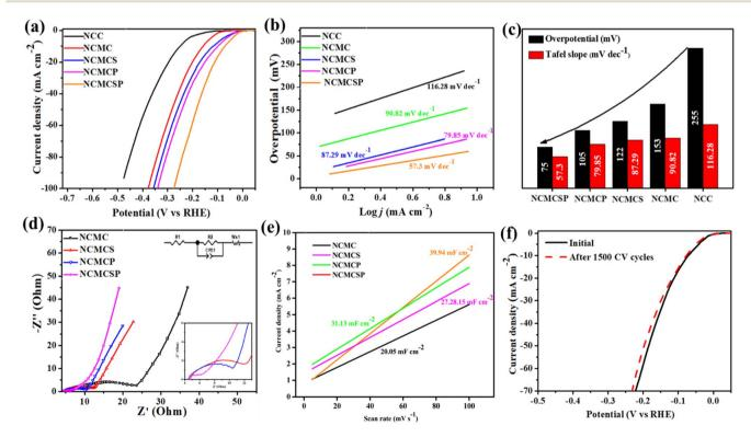
Fig. 5 (a) HER polarization curves, (b) Tafel curves in  $0.5 \,\mathrm{M}\,\mathrm{H}_2\mathrm{SO}_4$ , (c) comparison of overpotentials and Tafel slopes, (d) Nyquist plots, (e) double layer capacitance curves, and (f) HER polarization curves before and after 1500 CV cycles.
