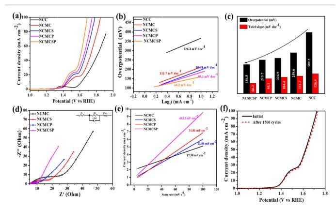
Fig. 7 (a) OER polarization curves, (b) the corresponding Tafel curves, (c) comparison of overpotential values and Tafel slopes, (d) Nyquist plots, (e) double layer capacitance curves, and (f) OER polarization curves for NCMCSP before and after 1500 CV cycles.
