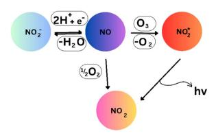
Fig. 2 Gas-phase chemiluminescence.
