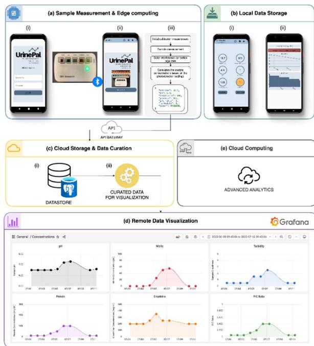
Fig. 5 Scheme representing data architecture (a–e) in POC nitrite sensing systems (reproduced from: V. S. Siu, M. Lu, K. Y. Hsieh, B. Wen, I. Buleje, N. Hinds, K. Patel, B. Dang and R. Budd, *Biosensors (Basel)*, 2024, 14), open access with permission from MDPI. Licensed under CC BY 4.0, 2024.
