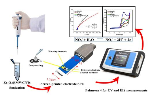
Fig. 4 Construction of a portable and disposable sensing system for the continuous monitoring of nitrite in food and environmental samples (reproduced from: N. Rajab, H. Ibrahim, R. Y. A. Hassan and A. F. A. Youssef, *RSC Advances*, 2023, **13**, 21259–21270), open access with permission from the Royal Society of Chemistry. Licensed under CC BY-NC 3.0, 2023.
