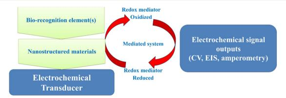
Scheme 3 Bio-electrochemical setup showing the main components including the transducer (electrode) modified with a layer of nanomaterial(s), followed by a layer of bio-recognition element(s) used for the selective analysis. The signal readouts could be obtained through the EIS, CV or/and amperometric techniques.
