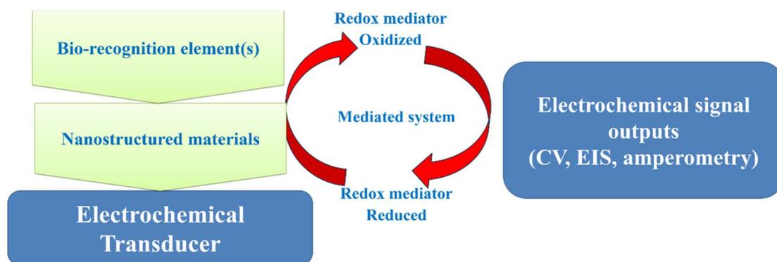
**Scheme 3** Bio-electrochemical setup showing the main components including the transducer (electrode) modified with a layer of nano-material(s), followed by a layer of bio-recognition element(s) used for the selective analysis. The signal readouts could be obtained through the EIS, CV or/and amperometric techniques.
