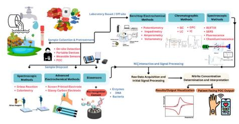
Scheme 1 Comprehensive overview of advanced instrumental methods for nitrite detection, illustrating their interconnections and diverse applications.
