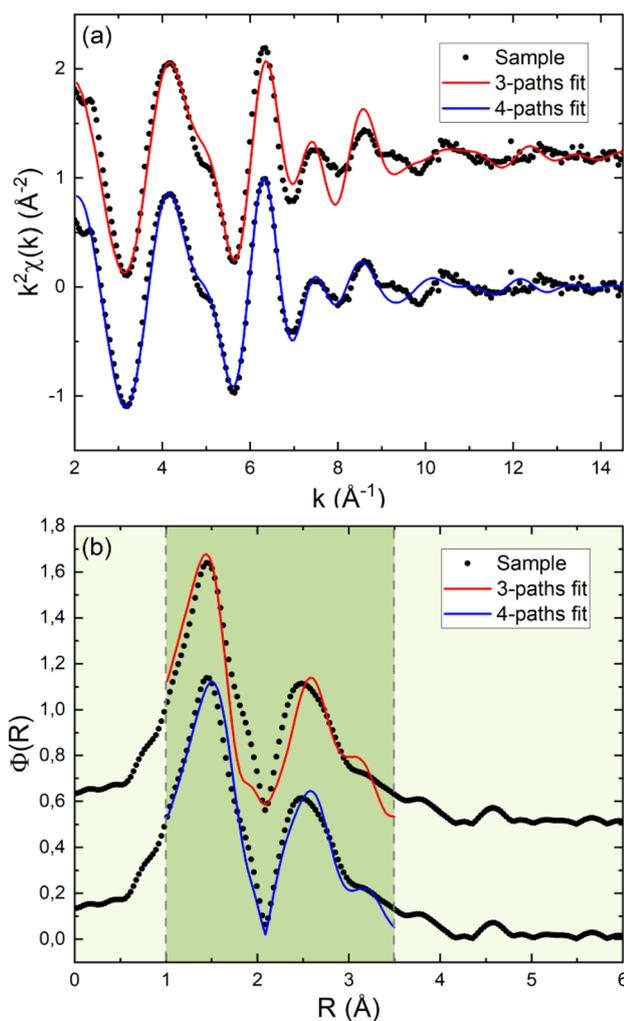
Fig. 4 (a) Room temperature  $k^2$ -weighted experimental EXAFS spectra and (b) the corresponding Fourier transform plot of the EXAFS signals shown in (a). Red and blue lines stand for a 3-path or 4-path fit, respectively.
