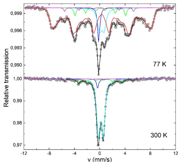
**Fig. 5** Mössbauer spectra together with the fit obtained at  $T = 300$  K and  $T = 77$  K. The grey dots and the solid black lines represent the experimental data and the fit, respectively. Different sub-spectra corresponding to Fe-oxides (red sextet and cyan doublet),  $\text{Fe}_3\text{C}$  (green sextet),  $\gamma\text{-Fe}$  (blue singlet) and  $\alpha\text{-Fe}$  (magenta sextet) phases have been considered.
