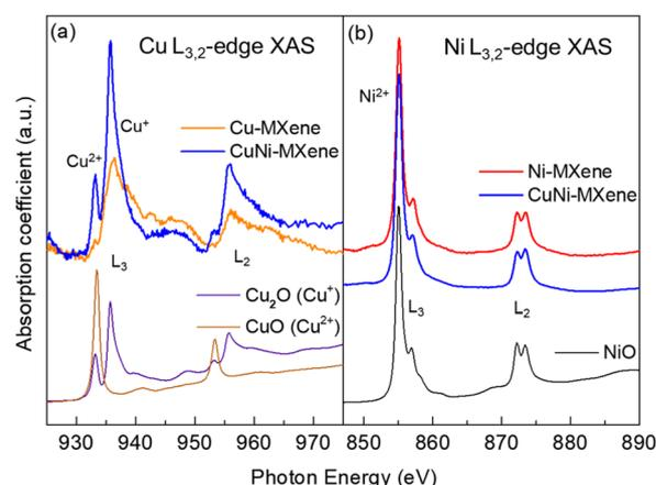
Fig. 3 (a) Cu L<sub>3,2</sub>-edge and (b) Ni L<sub>3,2</sub>-edge soft XAS spectra of the MXene samples together with reference spectra for comparison.
