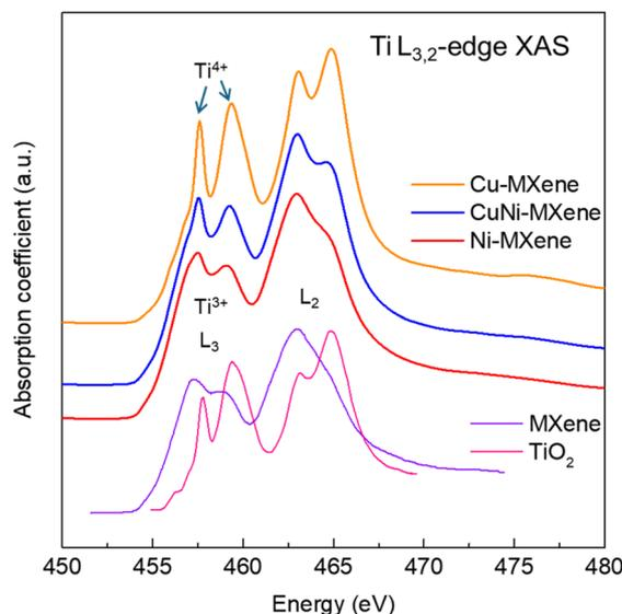
Fig. 4 Ti  $L_{3,2}$ -edge XAS spectra of the (Cu or Ni):MXene samples showing an evolution of Ti oxidation in accordance with the Cu incorporation. The spectra of pristine MXene and  $\text{TiO}_2$  are appended for comparison.
