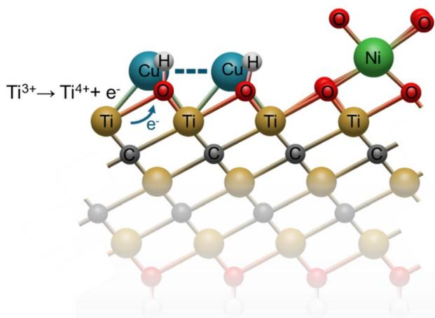
Fig. 1 Schematic for the atomic structure of a MXene nanosheet ( $\text{Ti}_3\text{C}_2\text{T}_x$ ) on which Cu or Ni ions are embedded, to demonstrate the chemical reaction of Ti ions invoked by active Cu ions and the resultant electron transfer to stabilize the  $\text{Cu}^{1+}$  ionic species.
