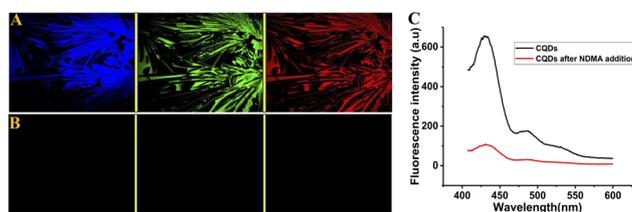
**Fig. 5** Fluorescence microscopy images of the thin film of the CQDs before (A) and after (B) NDMA addition, by subjecting the film to excitation at 405 nm with emission filter EM 450 (blue), excitation at 488 nm with emission filter EM 505 (green), and excitation at 543 nm with emission filter EM 595 (red). (C) Quenching of the fluorescence of a glass-supported solid film of the CQDs before and after the addition of NDMA.
