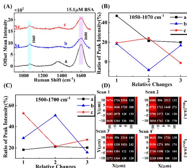
Fig. 4 UV-SERS on different samples a–c (black, blue and red spectra, respectively) with  $15.1\text{ }\mu\text{M}$  BSA and peak intensity analysis. (A) Mean intensity. (B–C) Ratios of peak intensity changes across four scans for Rh-modified Al ranging from  $1050$  to  $1070\text{ cm}^{-1}$  and  $1500$  to  $1700\text{ cm}^{-1}$ . (D) Mapping images of sample a across four scans in the range between  $1500$  and  $1700\text{ cm}^{-1}$ .
