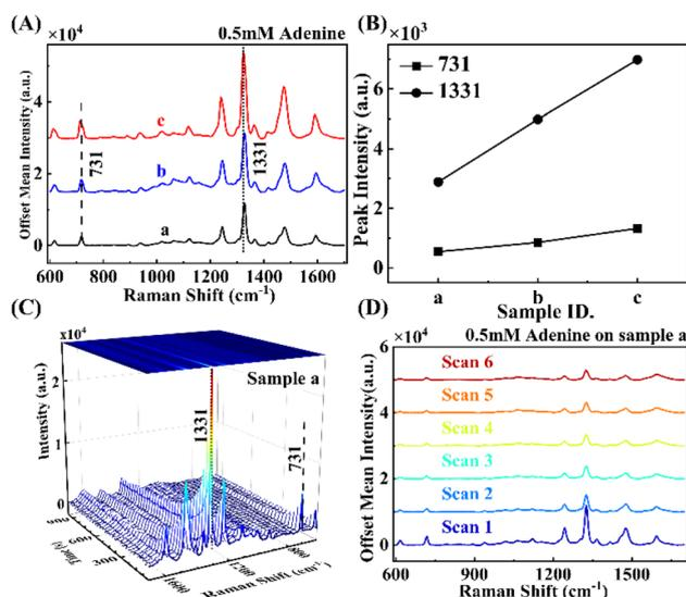
Fig. 2 Adenine UV-SERS spectra from Al–Rh NP samples. (A) Comparison between the first scans obtained from the three tested samples. (B) Maximum values around  $731 \text{ cm}^{-1}$  and  $1331 \text{ cm}^{-1}$  extracted from the spectra in (A). (C and D) 3D time-dependent SERS spectra and mean SERS spectra across six consecutive scans of 0.5 mM adenine on sample a.
