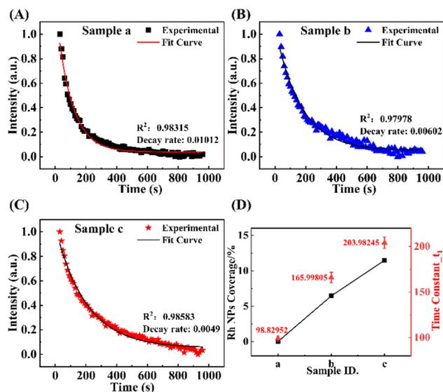
Fig. 3 (A–C) Experimental data and corresponding photodegradation fitting curves of peak intensity at around  $1331\text{ cm}^{-1}$  for adenine as a function of collection time for different samples a–c, respectively. (D) Time constants of sample a–c with varying Rh NPs coverage percentages.
