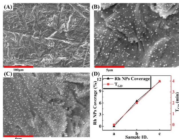
Fig. 1 Details of the prepared samples. SEM images of (A) untreated rough Al (sample a, no GD) and (B–C) Al samples subjected to galvanic displacement in 0.5 mM Na<sub>3</sub>RhCl<sub>6</sub>, pH 2.0, for different times: (B)  $t_{GD} = 2$  min (sample b); (C)  $t_{GD} = 4$  min (sample c), magnified detail. (D) Line chart depicting Rh NP coverage (%) for samples a–c at corresponding galvanic displacement times, showing 6.46% for sample b and 11.49% for sample c.
