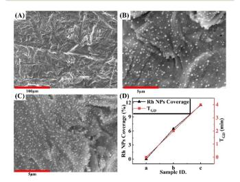
Fig. 1 Details of the prepared samples. SEM images of (A) untreated rough Al (sample a, no GD) and (B-C) Al samples subjected to galvanic displacement in 0.5 mM  $Na_3RhCl_6$ , pH 2.0, for different times: (B)  $t_{GD} =$ 2 min (sample b); (C)  $t_{GD} = 4$  min (sample c), magnified detail. (D) Line chart depicting Rh NP coverage (%) for samples a-c at corresponding galvanic displacement times, showing 6.46% for sample b and 11.49% for sample c.
