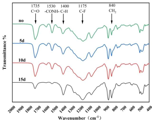
Fig. 4 FT-IR curves for PVDF/TPU/PC composite nanofibers.
