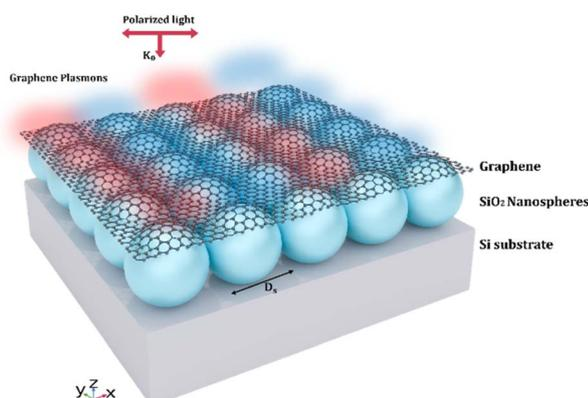
Fig. 1 Schematic demonstration of a deformed graphene structure on closely packed SiO<sub>2</sub> nanospheres with wrinkle period  $D_s$  on a silicon substrate. Polarized light with the electric field along the wrinkling directions  $x$  and  $y$  irradiates in the normal direction  $K_0$  to the structure to excite graphene plasmons.
