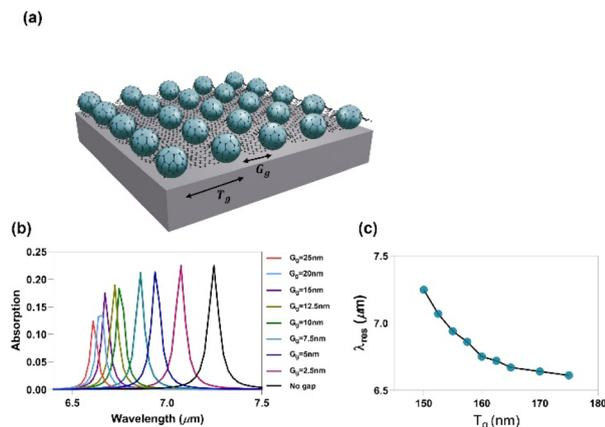
Fig. 5 (a) Schematic demonstration of a biaxially deformed graphene structure on the SiO<sub>2</sub> nanospheres with a graphene gap  $G_g$  and wrinkle period  $T_g = D_s + G_g$ . (b) Optical absorption spectra for the wrinkled graphene structure with varying  $G_g$  from 0 to 25 nm at  $D_s = 150$  nm. (c) Scaling of the fundamental-mode resonant wavelength with respect to wrinkle period  $T_g$ .
