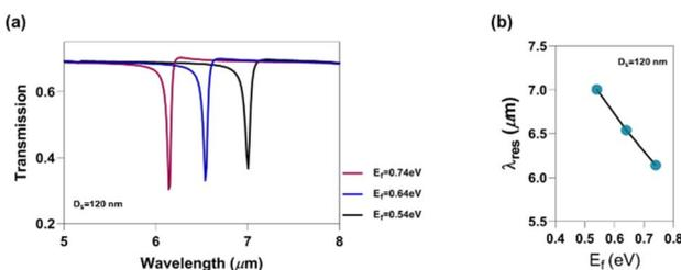
**Fig. 7** (a) Normal-incidence transmission spectra of biaxially corrugated graphene structures on the close-packed SiO<sub>2</sub> nanospheres with different Fermi energy levels  $E_f$  in graphene when  $D_s = 120$  nm. (b) Scaling of the fundamental-mode resonant wavelength with respect to  $E_f$ .
