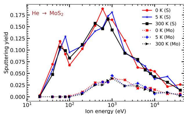
Fig. 4 Sputtering yields of Mo and S atoms from a free-standing  $\text{MoS}_2$  monolayer as functions of He ion energy at various temperatures (0, 5, and 300 K).
