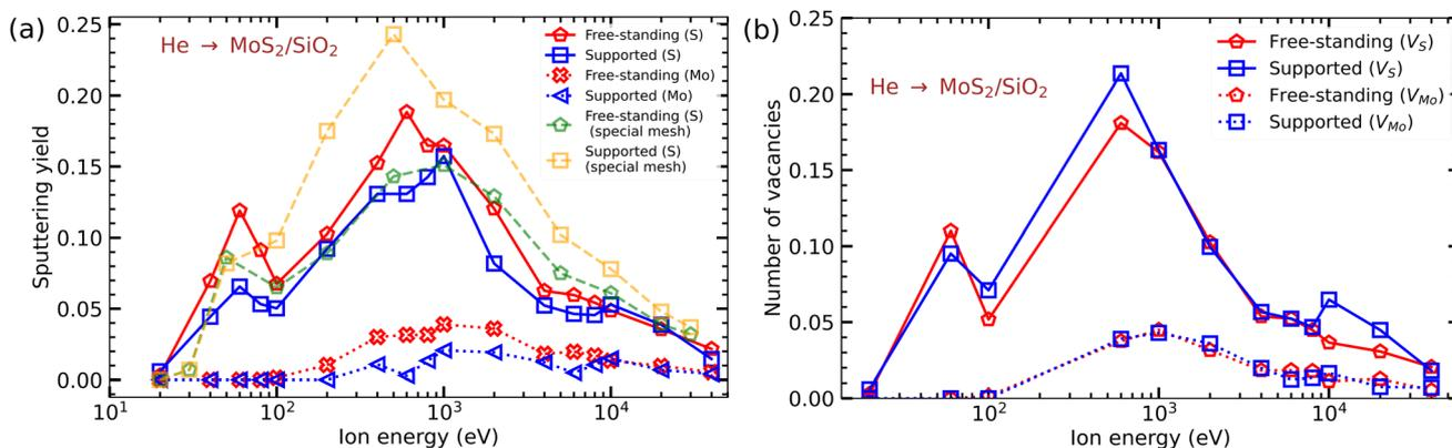
Fig. 6 (a) Mo and S atoms sputtering yields from a free-standing MoS<sub>2</sub> monolayer on a SiO<sub>2</sub> substrate as functions of He ion energy. (b) The number of Mo and S vacancies produced in the system per ion impact as a function of He ion energy.
