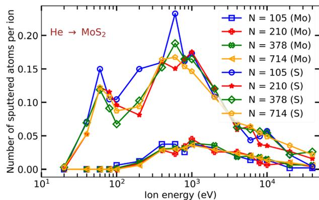
Fig. 3 Average number of S and Mo atoms sputtered from a free-standing  $\text{MoS}_2$  sheet upon impacts of He ions as functions of He ion energy calculated using different numbers of impact points  $N$ .
