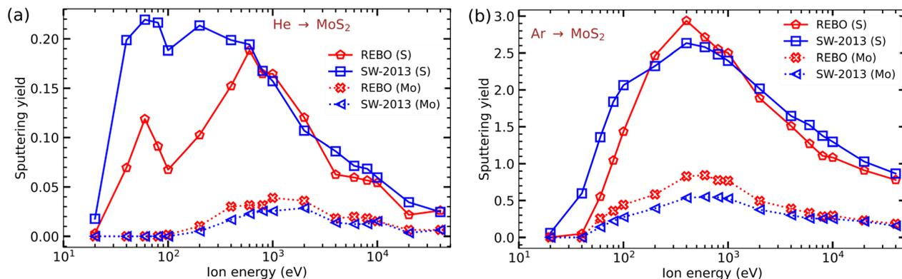
Fig. 5 Sputtering yields of Mo and S atoms from a free-standing MoS<sub>2</sub> monolayer calculated as functions of ion energy for (a) He and (b) Ar ions using the SW and REBO potentials.
