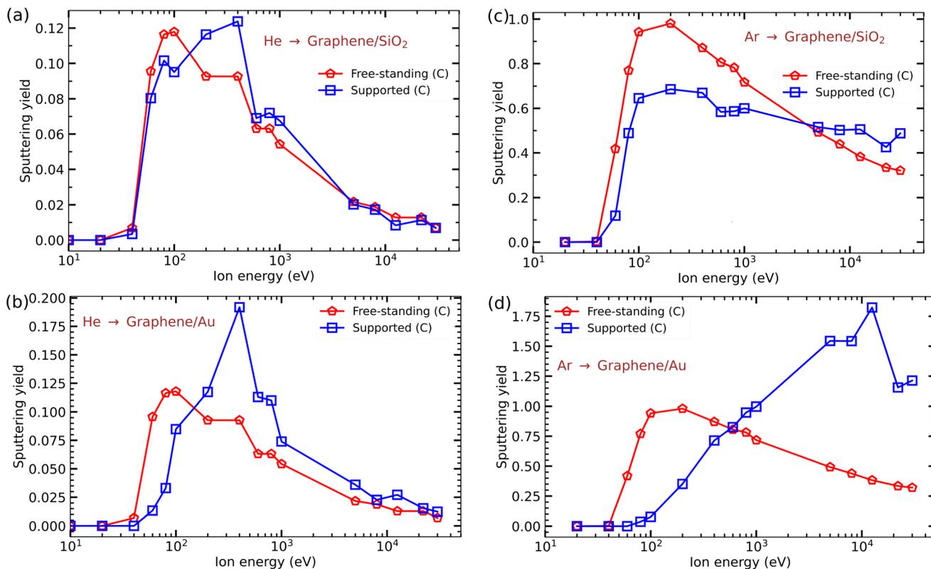
Fig. 9 Sputtering yields of C atoms from suspended and supported graphene as functions of He and Ar ion energies. (a) Impacts of He ions onto graphene on the SiO<sub>2</sub> substrate. (b) Impacts of He ions onto graphene on the Au substrate. (c) Impacts of Ar ions onto graphene on the SiO<sub>2</sub> substrate. (d) Impacts of Ar ions onto graphene on the Au substrate.
