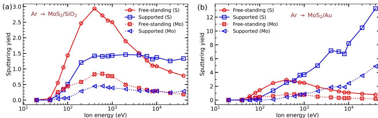
Fig. 8 Sputtering yields of Mo and S atoms as functions of Ar ion energies for suspended MoS<sub>2</sub> and MoS<sub>2</sub> on the SiO<sub>2</sub> substrate (a) and Au substrate (b).
