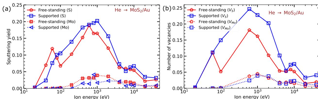
Fig. 7 (a) Sputtering yields of Mo and S atoms from free-standing and MoS<sub>2</sub> on the Au (111) substrate per as functions of He ion energy. (b) The number of Mo and S vacancies produced in the system per ion impact as a function of He ion energy.
