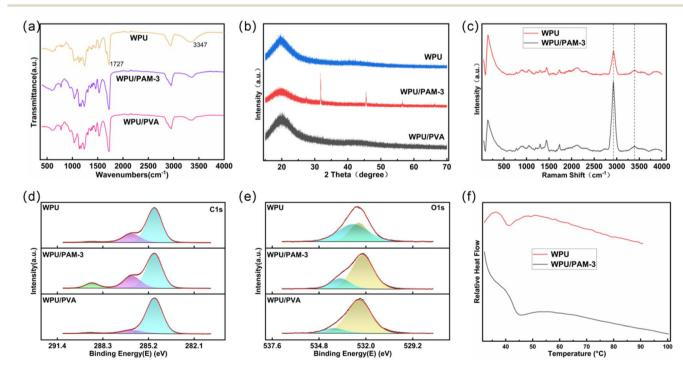
Fig. 3 (a) FTIR spectra of WPU, WPU/PAM-3, and WPU/PVA nanofiber membranes. (b) XRD patterns of WPU, WPU/PAM-3, and WPU/PVA membranes. (c) Raman spectra of WPU and WPU/PAM-3 nanofibers. (d) High-resolution C 1s XPS spectra of WPU, WPU/PAM-3, and WPU/PVA. (e) High-resolution O 1s XPS spectra of WPU, WPU/PAM-3, and WPU/PVA. (f) DSC curves of WPU and WPU/PAM-3 nanofibers
