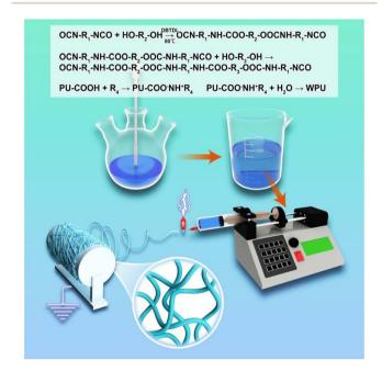
Fig. 1 Schematic of the synthesis and electrospinning process of WPU nanofibers.
