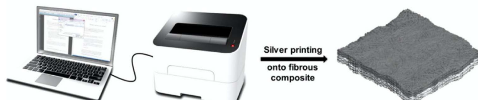
Fig. 14 Steps of the electro-spun membrane printing process. The image is reproduced from a previous study 137 with permission from Elsevier.
