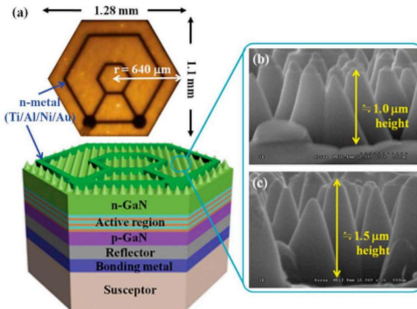
Fig. 12 Honeycomb-type VLED with a textured cone-shaped deep-pillar surface.<sup>125</sup>
