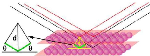
Fig. 3 Conditions for the Bragg diffraction of light on a PC structure: constructive interference between adjacent crystal planes.<sup>35</sup>
