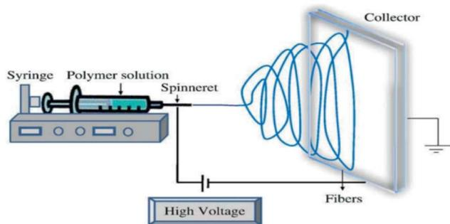
**Experimental set-up of electrospinning.** The 3D printing technology for fabricating the whole membrane is still under development. However, more realistic studies based on current technology can be seen in research regarding the inkjet printing or 3D printing of solvents or gels on the surface of membranes.
