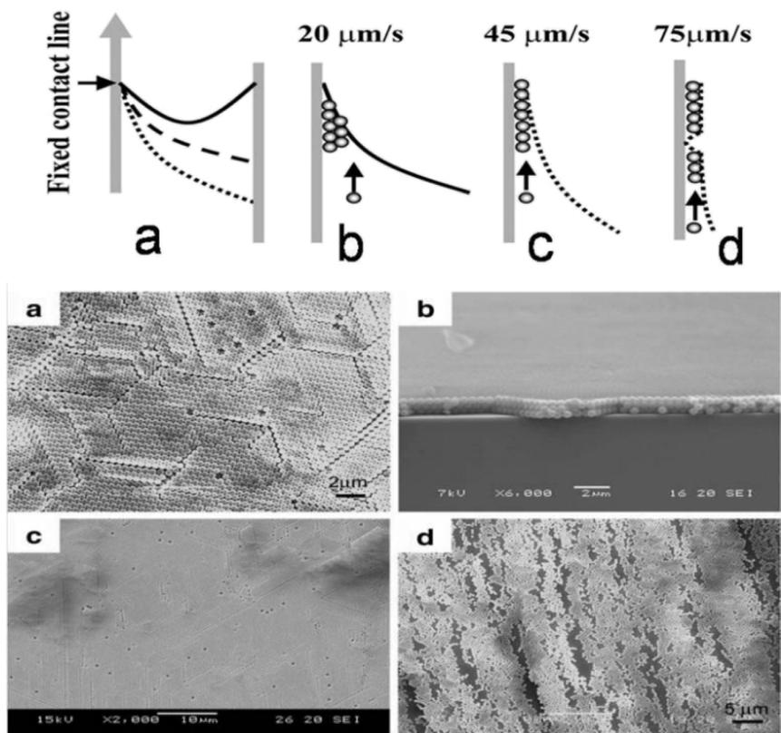
Fig. 9 Meniscus lift-up observed at different contact line speeds. The top panel shows schematic shapes of the meniscus at lift-up rates of  $20 \mu\text{m s}^{-1}$ ,  $45 \mu\text{m s}^{-1}$ , and  $75 \mu\text{m s}^{-1}$ . The bottom panel presents SEM images of the corresponding colloidal crystals: (a)  $20 \mu\text{m s}^{-1}$ ; (b) side view of a tri-layer at  $20 \mu\text{m s}^{-1}$ ; (c)  $45 \mu\text{m s}^{-1}$ ; (d)  $75 \mu\text{m s}^{-1}$ . Reproduced from ref. 109.
