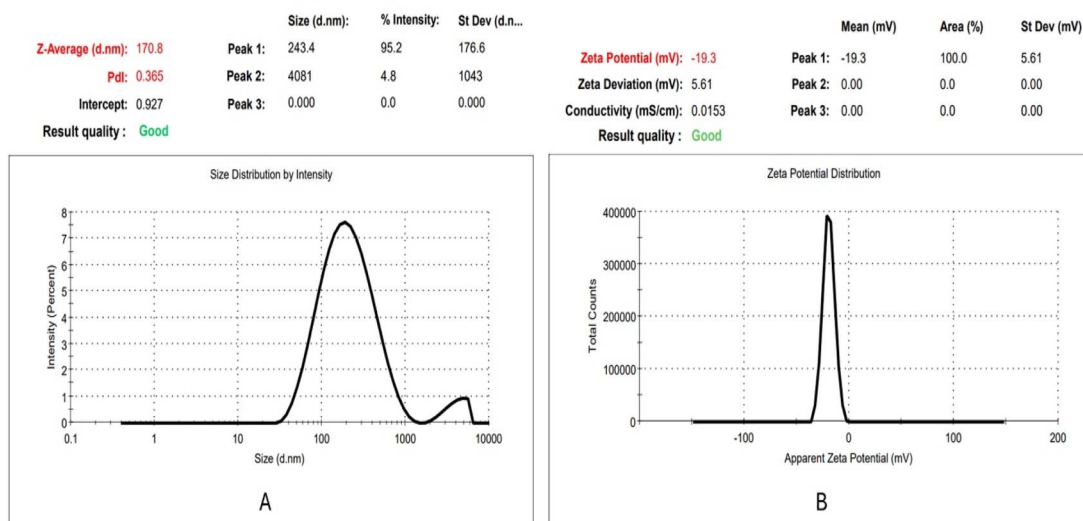
Fig. 7 (A) Particle size and PDI of optimized formulation; (B) zeta potential of optimized formulation.
