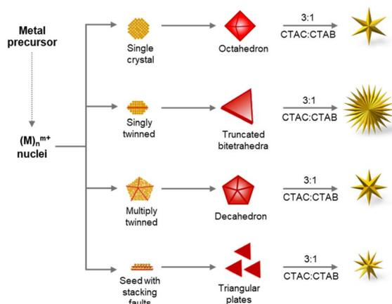
**Scheme 1** Schematic representation of the growth of our synthesized Au seeds with different defect structures and morphologies but the same {111} surface crystal facets. These Au NCs were subjected to overgrowth under identical synthetic conditions giving rise to stellated Au NCs.
