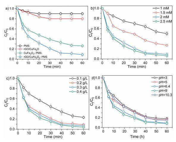
Fig. 8 (a) Removal efficiency of OG in different system, Reaction conditions:  $[catalyst] = 0.2 \text{ g L}^{-1}$ ; [PMS] = 2 mM;  $[OG] = 50 \text{ mg L}^{-1}$ ; initial pH without adjustment. Effects of operating parameters on OG degradation (b) PMS dosage, (c) catalyst dosage, and (d) various pH conditions.
