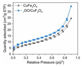
Fig. 4 Nitrogen adsorption/desorption isotherm of CuFe<sub>2</sub>O<sub>4</sub> and rGO/CuFe<sub>2</sub>O<sub>4</sub> samples.
