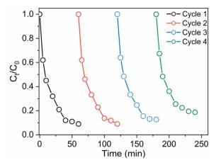
Fig. 11 Recycling tests of the rGO/CuFe<sub>2</sub>O<sub>4</sub> catalyst; reaction conditions:  $[catalyst] = 0.2 \text{ g L}^{-1}$ ; [PMS] = 2 mM; [OG] = 50
