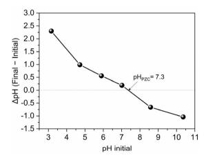
Fig. 9 pH point zero charge (pH<sub>P7C</sub>) of rGO/CuFe<sub>2</sub>O<sub>4</sub>.
