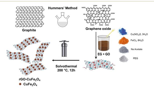
Fig. 1 Schematic illustration of the hydrothermal synthesis of rGO/CuFe<sub>2</sub>O<sub>4</sub> nanocomposite.
