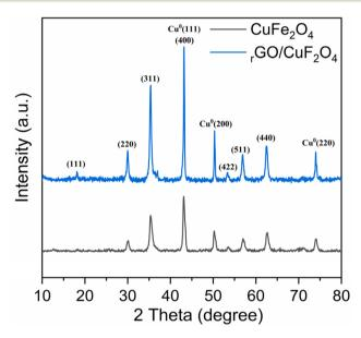
Fig. 2 XRD patterns of CuFe<sub>2</sub>O<sub>4</sub> and rGO/CuFe<sub>2</sub>O<sub>4</sub> samples.
