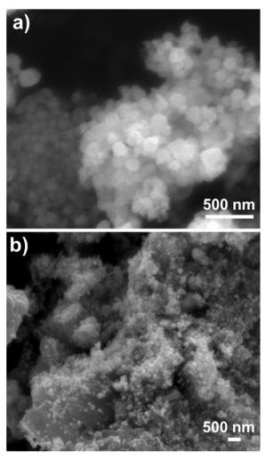
Fig. 5 SEM images of (a) CuFe<sub>2</sub>O<sub>4</sub> and (b) rGO/CuFe<sub>2</sub>O<sub>4</sub> samples.
