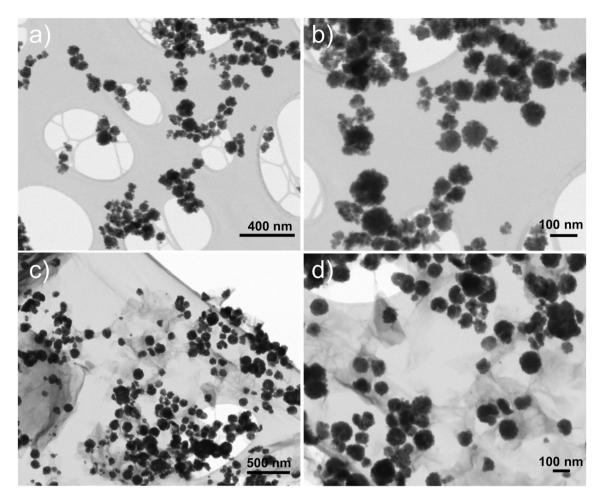
Fig. 6 STEM images of (a and b)  $CuFe_2O_4$  and (c and d)  $rGO/CuFe_2O_4$  samples.
