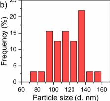
Fig. 7 Particle size distribution analysis of (a) CuFe $_2$ O $_4$  and (b) rGO/CuFe $_2$ O $_4$ .
