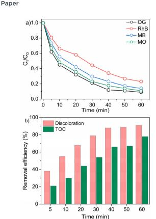
Fig. 10 (a) Degradation of various organic dyes using the rGO/ CuFe<sub>2</sub>O<sub>4</sub>-PMS system. (b) Discoloration and mineralization (TOC removal) of OG at different reaction times under optimal conditions. Reaction conditions:  $[catalyst] = 0.2 \text{ g L}^{-1}$ ; [PMS] = 2 mM; [OG] =50 mg  $L^{-1}$ , [BM] = 10 mg  $L^{-1}$ ; [RhB] = 10 mg  $L^{-1}$ ; [MO] = 10 mg  $L^{-1}$ .
