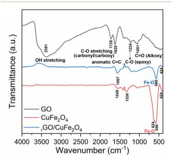
Fig. 3 FTIR spectra of graphene oxide (GO), CuFe $_2$ O $_4$  and rGO/CuFe $_2$ O $_4$  samples.
