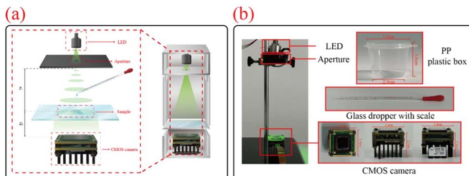
Fig. 1 Schematic diagram and set-up of the lensless holographic imaging experimental device; (a) schematic diagram of the lensless holographic imaging experimental device; (b) lensless holographic imaging experimental device and related material and equipment parameters.
