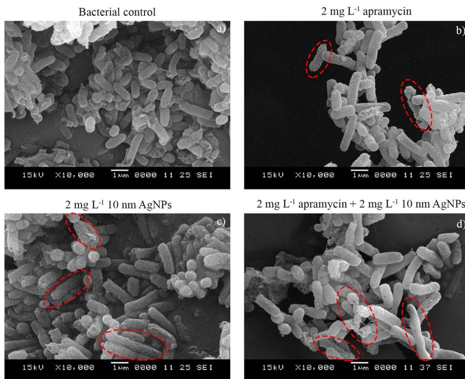
**Fig. 6** SEM images (10000 $\times$ ) of *E. coli* ATCC 25922: (a) control and exposed to (b)  $2 \text{ mg L}^{-1}$  apramycin, (c)  $2 \text{ mg L}^{-1}$  10 nm AgNPs and (d)  $2 \text{ mg L}^{-1}$  apramycin +  $2 \text{ mg L}^{-1}$  10 nm AgNPs.
