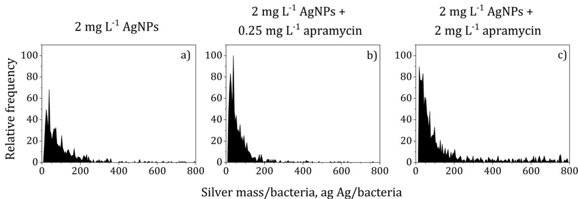
Fig. 4 Silver mass per bacteria distributions analysed by SC-ICP-MS for samples of *E. coli* ATCC 25922 bacteria exposed to: (a) 2 mg L<sup>-1</sup> AgNPs, (b) 2 mg L<sup>-1</sup> AgNPs + 0.25 mg L<sup>-1</sup> apramycin and (c) 2 mg L<sup>-1</sup> AgNPs + 2 mg L<sup>-1</sup> apramycin.
