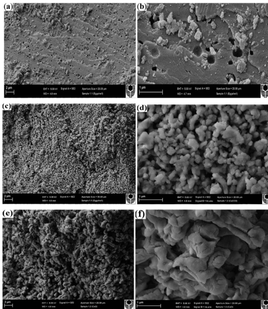
Fig. 5 SEM images of the eggshell (a and b) as-crushed and calcined at: (c and d) 600 and (e and f) 900 °C. This figure has been adapted/reproduced from ref. 95 with permission from *RSC Adv.*, copyright 2019.
