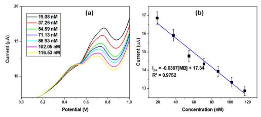
Fig. 15 (a) SWV of  $Au_{qrn}/MWCNTs$  in MB concentration ranging from 19.08 to 116.53 nm and (b)  $Au_{chm}/MWCNT$  linear plot of  $I_p$  vs. conc.
