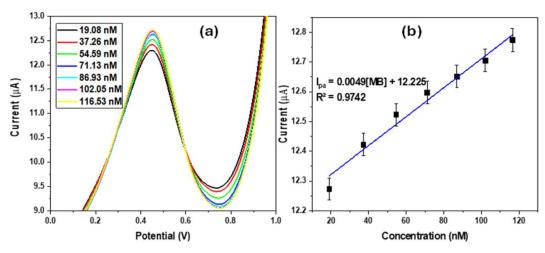
Fig. 14 (a) SWV of Au<sub>chm</sub>/MWCNTs in MB concentration ranging from 19.08 to 116.53 nm and (b) Au<sub>chm</sub>/MWCNT linear plot of I<sub>p</sub> vs. conc.
