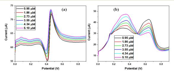
Fig. 16 (a) SWV of Au<sub>chm</sub>/MWCNTs detecting MB (0.5 V) in the presence of SSY (0.1 and 0.2 V) and (b) Au<sub>chm</sub>/MWCNTs detecting MB (0.65 V) in the presence of SSY (0.3 V).
