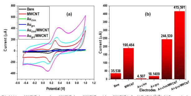
Fig. 7 CV of (a) bare, MWCNT,  $Au_{chm}$ ,  $Au_{grn}$ , MWCNT,  $Au_{chm}$ /MWCNT, and  $Au_{grn}$ /MWCNT in 5 mM [Fe(CN)<sub>6</sub>]<sup>3-/4-</sup>. (b) Bar graph of oxidation peaks of all electrodes.
