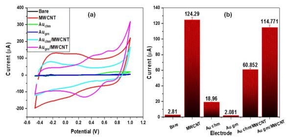
Fig. 11 CV of (a) bare, MWCNTs,  $Au_{chm}$ ,  $Au_{grn}$ , MWCNTs,  $Au_{chm}$ /MWCNTs, and  $Au_{grn}$ /MWCNTs in MB (0.1 mM). (b) Bar graph of oxidation peaks of modified and unmodified electrodes.
