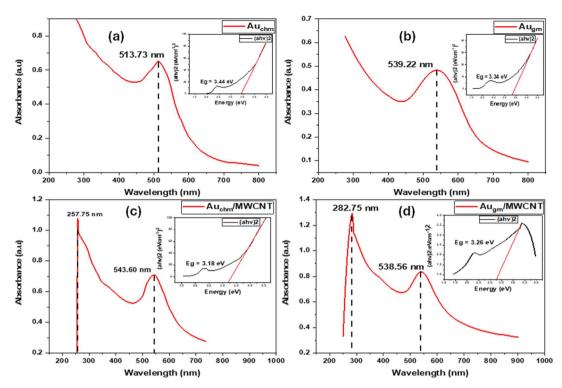
Fig. 1 The optical absorption spectra of (a)  $Au_{chm}$ , (b)  $Au_{grn}$ , (c)  $Au_{chm}$ /MWCNTs, and (d)  $Au_{grn}$ /MWCNTs. The inserted images are the Tauc plots for each nanomaterial.
