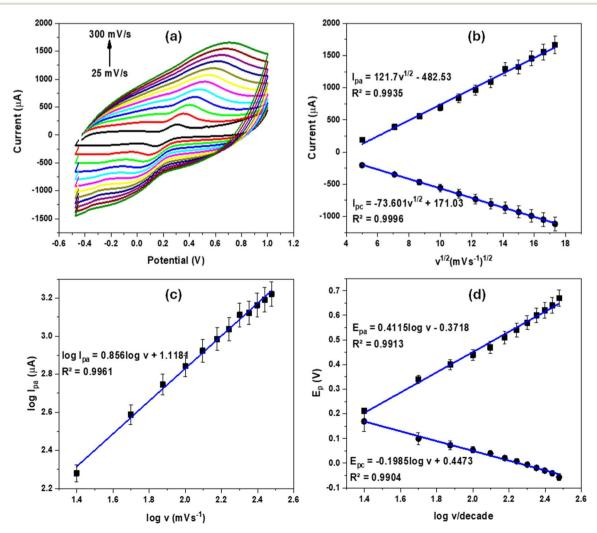
Fig. 10 (a) The scan rate of  $Au_{qrn}/MWCNTs$ , (b)  $I_p$  vs.  $v^2$ , (c)  $\log I_{pa}$  vs.  $\log v$ , and (d)  $E_p$  vs.  $\log v$  in 5 mM [Fe(CN)<sub>6</sub>]<sup>3-/4-</sup>.
