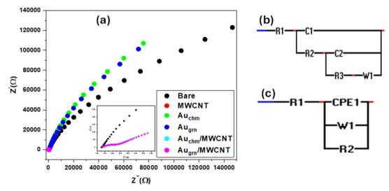
Fig. 8 (a) Nyquist plot of all the nanomaterials and (b and c) equivalent circuit models.
