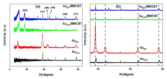
Fig. 3 XRD diffractograms of (a) Au<sub>chm</sub>, Au<sub>grn</sub>, MWCNTs, Au<sub>chm</sub>/MWCNTs, and Au<sub>grn</sub>/MWCNTs. (b) Magnified view of (a) from 35 to 80°.
