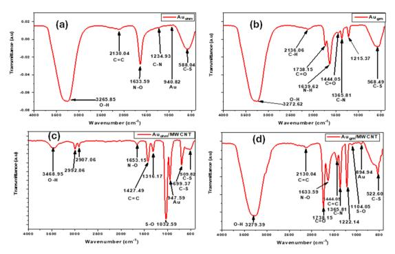
Fig. 2 The functional groups of (a) Au<sub>chm</sub>, (b) Au<sub>grn</sub>, (c) Au<sub>chm</sub>/MWCNTs, and (d) Au<sub>grn</sub>/MWCNTs in FTIR spectra.
