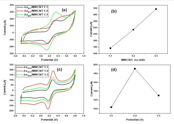
Fig. 6 Electrode optimization study of (a and b) Au<sub>chm</sub>: MWCNT and (c and d) Au<sub>grn</sub>: MWCNT.
