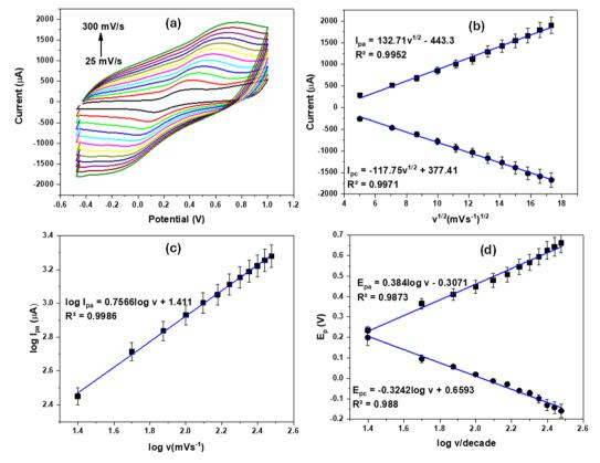
Fig. 9 (a) The scan rate of Au<sub>chm</sub>/MWCNTs, (b)  $I_p$  vs.  $v^2$ , (c)  $\log I_{pa}$  vs.  $\log v$ , and (d)  $E_p$  vs.  $\log v$  in 5 mM [Fe(CN)<sub>6</sub>]<sup>3-/4-</sup>.
