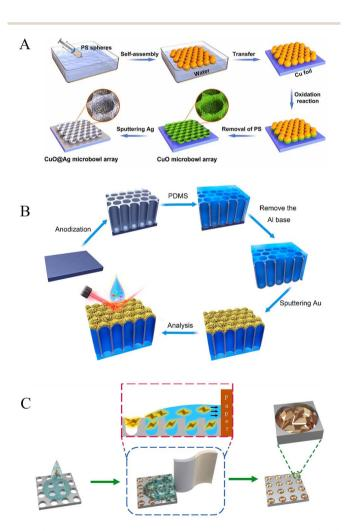
Fig. 3 Schematic illustrations for the preparation of partial solid SERS substrates. (A) Illustrates the process of constructing SERS substrates by direct deposition of colloidal nanoparticles onto solid substrates.55 (B) and (C) show the preparation procedures for constructing SERS substrates via template-assisted methods. 56,57
