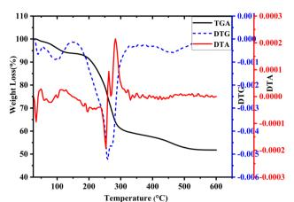
Fig. 13 TGA, DTG and DTA of Ag@SiO<sub>2</sub>-SO<sub>3</sub>H.
