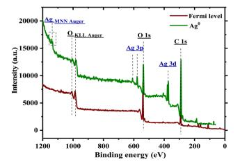
Fig. 12 XPS survey scan (spectra) of the AgNPs and valence band spectra in the vicinity of the Fermi level.
