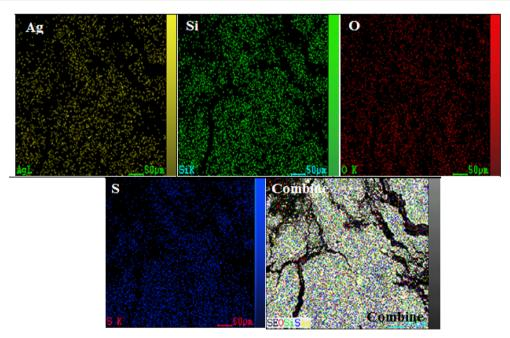
Fig. 4 SEM-coupled EDX (SEM mapping) of Ag@SiO<sub>2</sub>-SO<sub>3</sub>H.
