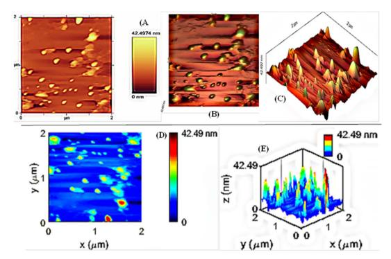
Fig. 7 AFM topography images of  $Ag@SiO_2-SO_3H$  in dimensions of  $2 \times 2$  microns. (A) initial image, (B) 2D image, (C) 3D image, (D) improved 2D image in Mat lab with color bar, (E) improved 3D image in Mat lab with color bar.
