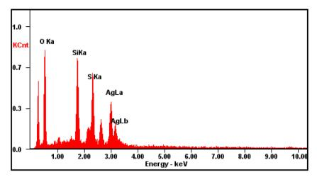
Fig. 3 EDX analysis of Ag@SiO<sub>2</sub>-SO<sub>3</sub>H.
