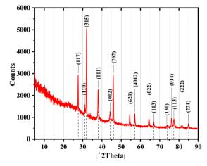
Fig. 10 XRD pattern of the Ag@SiO<sub>2</sub>-SO<sub>3</sub>H.
