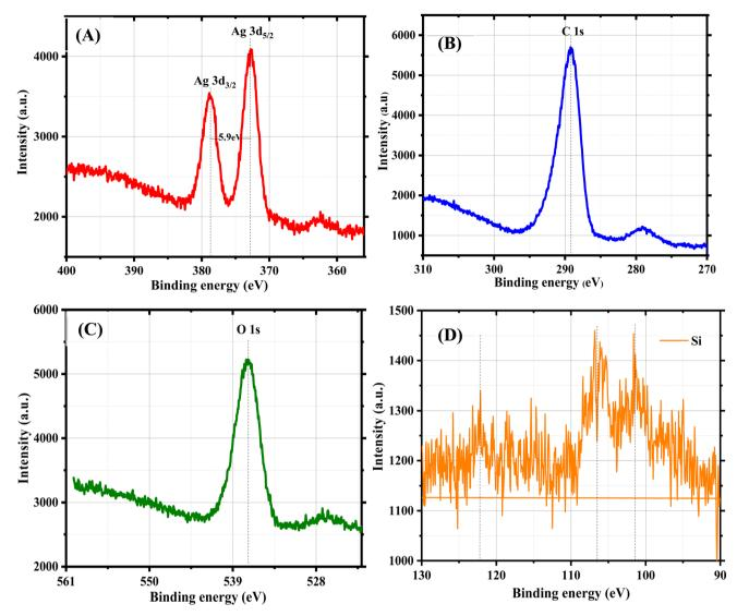
Fig. 11 High-resoluotion XPS spectra: (A) 3d Ag, (B) 1s C, (C) 1s O, (D) Si.
