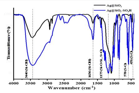
Fig. 2 FT-IR spectra of Ag@SiO<sub>2</sub>-SO<sub>3</sub>H and Ag@SiO<sub>2</sub> nanoparticles.
