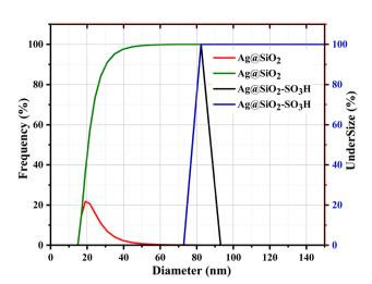
Fig. 5 Comparison of DLS of Ag@SiO<sub>2</sub> and Ag@SiO<sub>2</sub>-SO<sub>3</sub>H.
