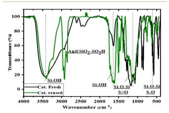
Fig. 16 FT-IR spectra of the fresh and reused Ag@SiO<sub>2</sub>-SO<sub>3</sub>H.
