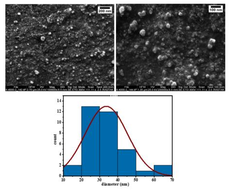
Fig. 8 FE-SEM images (micrographs) of the Ag@SiO<sub>2</sub>-SO<sub>3</sub>H.
