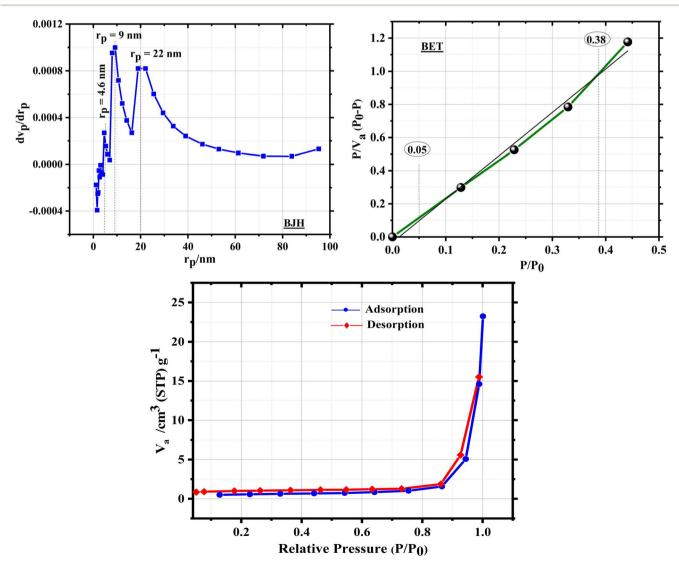
Fig. 14 BJH, BET and adsorption and desorption isotherms for the Ag@SiO<sub>2</sub>-SO<sub>3</sub>H.
