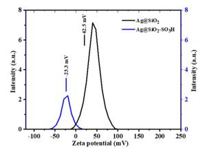
Fig. 6 Comparison of the zeta potentials of Ag@SiO<sub>2</sub> and Ag@SiO<sub>2</sub>-SO<sub>3</sub>H.
