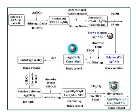
Fig. 1 Preparation of Ag@SiO<sub>2</sub>-SO<sub>3</sub>H.
