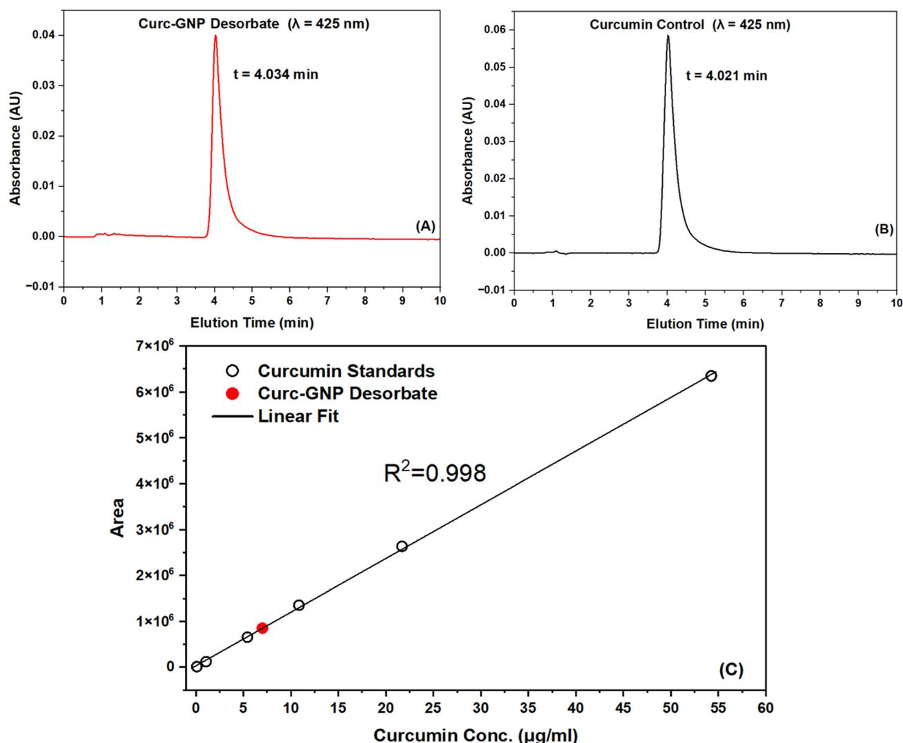
Fig. 4 HPLC analysis of curcumin loading. (A) Chromatogram of Curc-GNP desorbate ( $t = 4.034 \text{ min}$ ). (B) Chromatogram of curcumin control ( $t = 4.02 \text{ min}$ ). (C) Calibration curve for curcumin ( $0.1\text{--}55 \mu\text{g mL}^{-1}$ ;  $R^2 = 0.998$ ) with Curc-GNP desorbate plotted in red.
