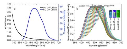
Fig. 3 (a) Absorption and emission spectra of the blue fluorescent CNPs ( $\lambda_{\rm exc} = 370$  nm and  $\lambda_{\rm em} = 475$  nm); (b) normalized excitation-dependent emission spectra of DMSO dispersed CNPs, [CNPs] = 0.2 mg mL<sup>-1</sup>, with the inset showing the blue, yellow and green emitting CNPs under the excitation of 350 nm, 427 nm and 520 nm wavelengths, respectively.
