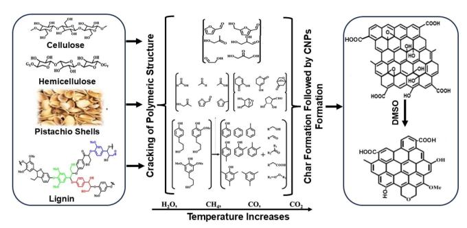
Scheme 2 Possible mechanism of the development of CNPs via the ultrasonication of pistachio shell-derived biochar.
