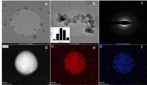
Fig. 1 HRTEM images of CNPs: (a) low magnification; (b) high magnification with a particle size distribution plot in the inset; (c) the SAED pattern showing a dull ring and (d-f) HADF mapping of carbon and oxygen, respectively.
