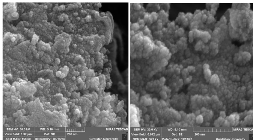
Fig. 4 SEM images of Pd@boehmite.
