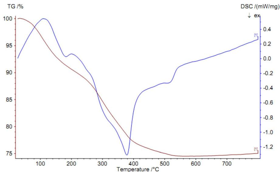
Fig. 3 TGA and DSC diagrams of Pd@boehmite.
