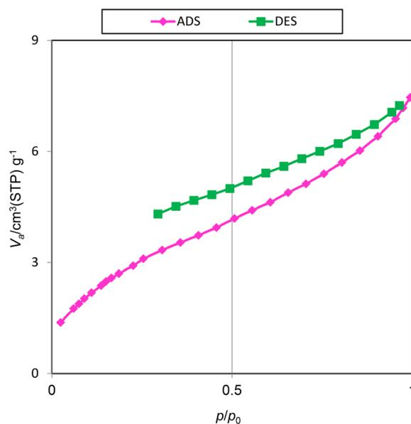
Fig. 2 N<sub>2</sub> adsorption-desorption isotherms of Pd@boehmite.
