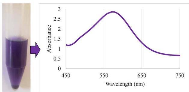
Fig. 1 UV spectrum after a ninhydrin test for NH<sub>2</sub>@boehmite.
