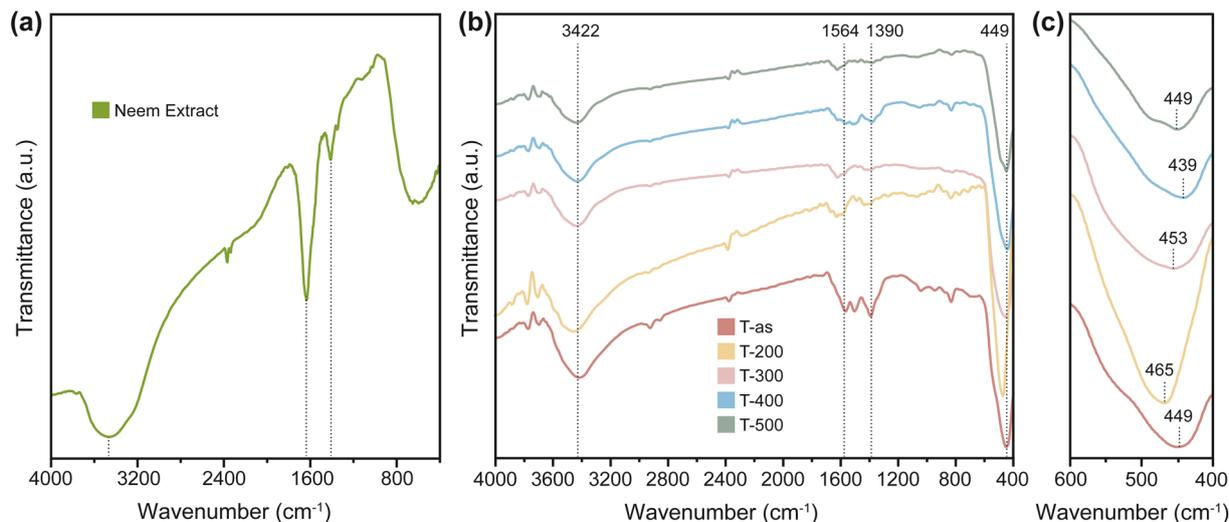
Fig. 3 FTIR spectra of (a) the leaf extract of *Azadirachta indica* representing the presence of bioactive compounds and (b) ZnO NPs annealed at different temperatures. The magnified view (c) of the spectra displays the peak shift of Zn–O due to temperature variation.
