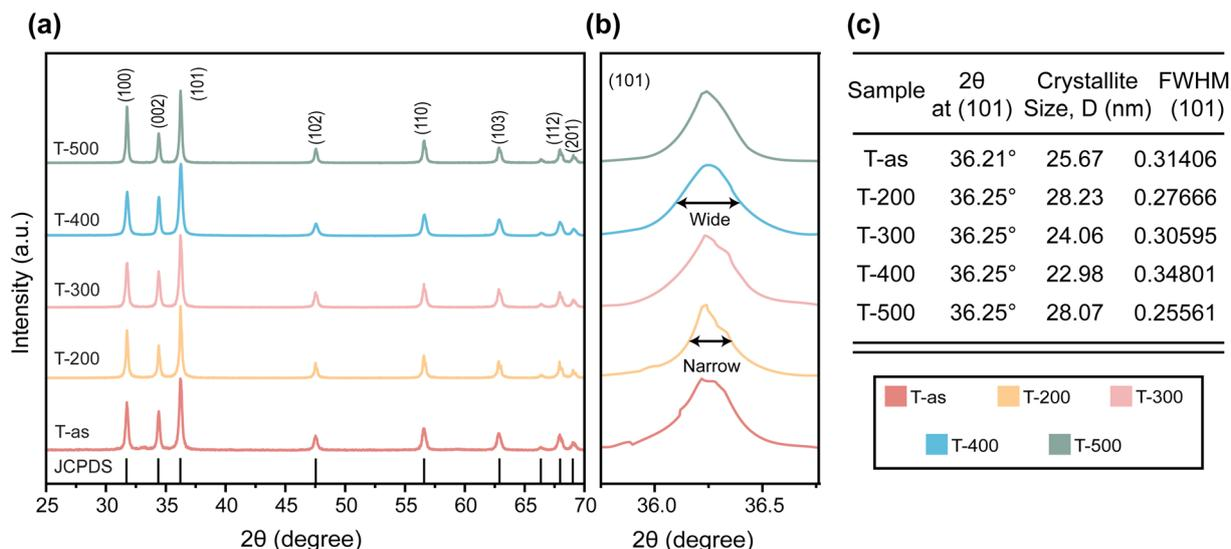
Fig. 4 (a) X-ray diffraction patterns of different ZnO NP samples, (b) XRD peaks at (101) spectra of ZnO NPs synthesized using *Azadirachta indica* leaf extract and annealed at different temperatures, highlighting structural changes, and (c) a table containing average crystallite size and FWHMs of different ZnO NP samples.
