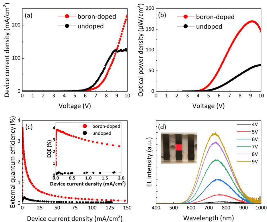
Fig. 3 Comparison of the device characteristics of B-doped and undoped Si-QLEDs: (a)  $I$ - $V$  characteristics, (b) optical power density as a function of voltage, (c) plots of EQE as a function of device current density (the inset shows a zoomed-in view of the EQE dependence at current densities between 0 and 2 mA cm<sup>-2</sup>) and (d) EL spectra of B-doped Si-QLEDs plotted at different applied voltages. The insets show a photograph of the device operating at 9 V.
