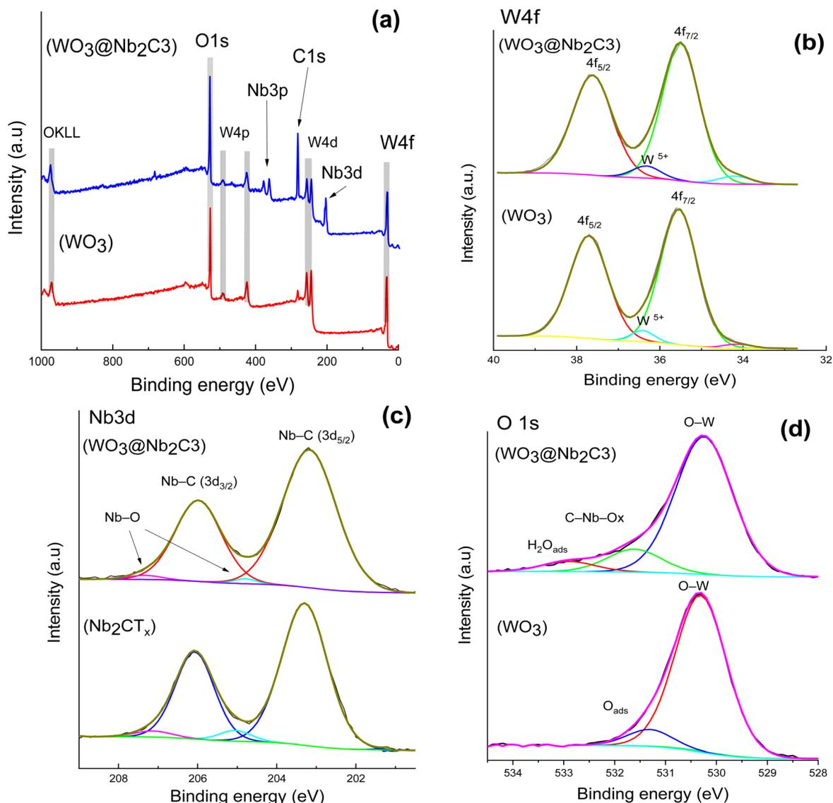
Fig. 3 XPS survey scan of  $\text{WO}_3$  and  $\text{WO}_3@Nb_2C_3$  (a); high resolution XPS spectra of W 4f of  $\text{WO}_3$  and  $\text{WO}_3@Nb_2C_3$  (b); high resolution XPS spectra of Nb 3d of  $Nb_2CT_x$  and  $\text{WO}_3@Nb_2C_3$  (c); and high resolution XPS spectra of O 1s of  $\text{WO}_3$  and  $\text{WO}_3@Nb_2C_3$  (d).
