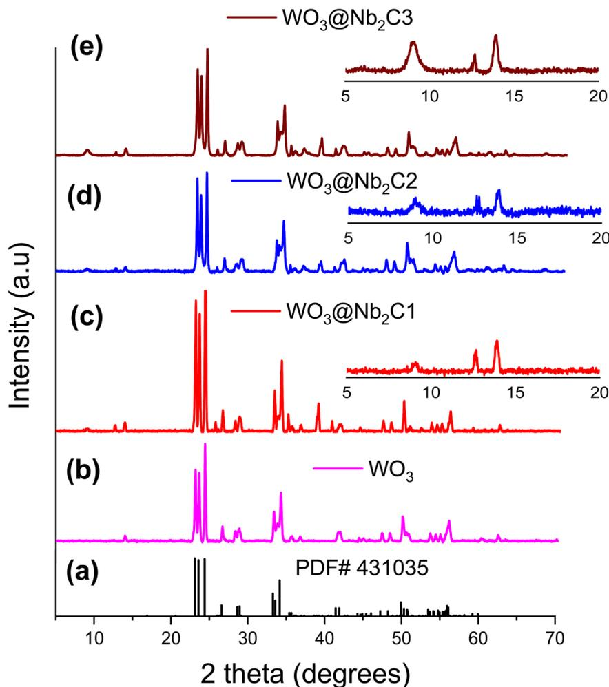
Fig. 2 XRD patterns of the  $\text{WO}_3$  reference card (a),  $\text{WO}_3$  (b),  $\text{WO}_3@Nb_2C_1$  (c),  $\text{WO}_3@Nb_2C_2$  (d), and  $\text{WO}_3@Nb_2C_3$  (e). The insets show the magnified patterns of (c)–(e).
