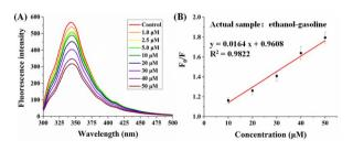
Fig. 6 (A) Fluorescence spectra of CA-CDs with different concentrations of Fe<sup>3+</sup> in automotive ethanol gasoline and (B) the corresponding plot of the relative quenching efficiency  $(F_0/F)$  against the concentration of Fe3-
