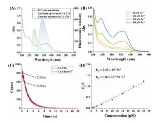
Fig. 7 (A) UV-vis absorption spectrum of Fe<sup>3+</sup>-ethanol solution (red line) and the excitation/emission spectra of CA-CDs (green/black line). (B). UV-vis absorption spectra of different concentrations of Fe<sup>3+</sup> in ethanol. (C) Fluorescence lifetime investigation of CA-CDs in the absence (black line) and presence (red line) of Fe<sup>3+</sup>. (D) The quenching constant ( $K_{sv}$ ) and bimodular quenching constant ( $K_{q}$ ) calculated using the Stern-Volmer equation.
