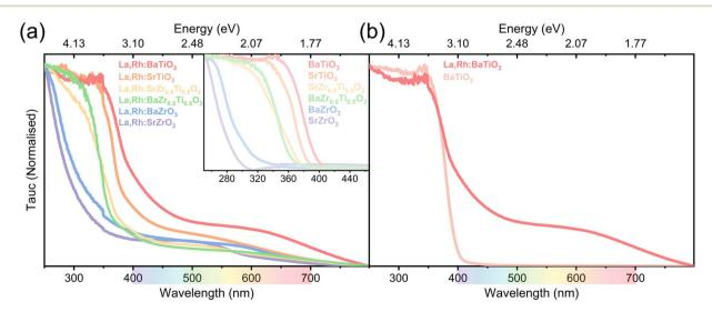
Fig. 3 (a) Normalised Tauc plot of La,Rh:ABO<sub>3</sub> perovskites. The inset contains Tauc plots for the base perovskites. (b) The Tauc of La,Rh codoped and undoped BTO are plotted to demonstrate the visible light absorption conferred by La,Rh co-doping
