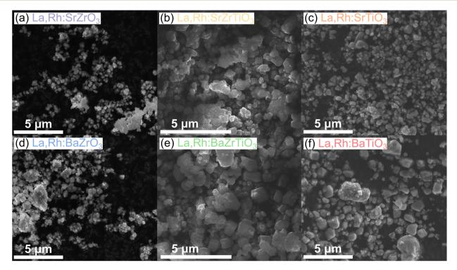
Fig. 5 SEM images of La,Rh co-doped perovskites. (a) La,Rh:SrZrO<sub>3</sub>. (b) La,Rh:SrZrTiO<sub>3</sub>. (c) La,Rh:SrTiO<sub>3</sub>. (d) La,Rh:SrZrO<sub>3</sub>. (e) La,Rh:SrZrTiO<sub>3</sub>. (f) La,Rh:SrTiO<sub>3</sub>.
