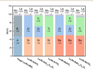
Fig. 4 ICP-MS derived mol% of elements comprising the La,Rh:ABO<sub>3</sub> perovskites. The corresponding stoichiometry is labelled in black (normalised to the A element, Sr or Ba).
