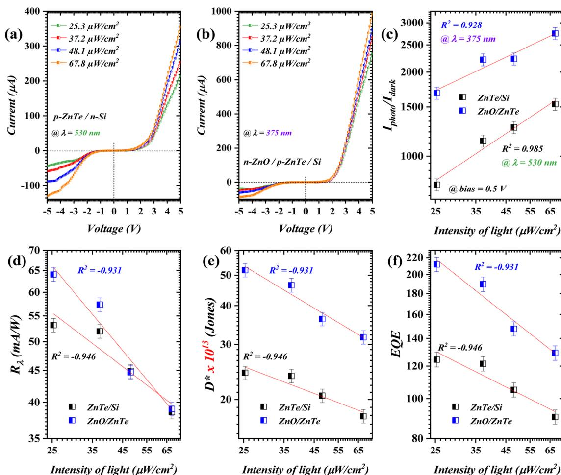
Fig. 4 Incident power density dependency of  $I$ - $V$  characteristics of (a) p-ZnTe/n-Si and (b) n-ZnO/p-ZnTe/Si, with figure-of-merits are presented in (c)  $I_{\text{photo}}/I_{\text{dark}}$ , (d)  $R_\lambda$ , (e)  $D^*$ , and (f) EQE.
