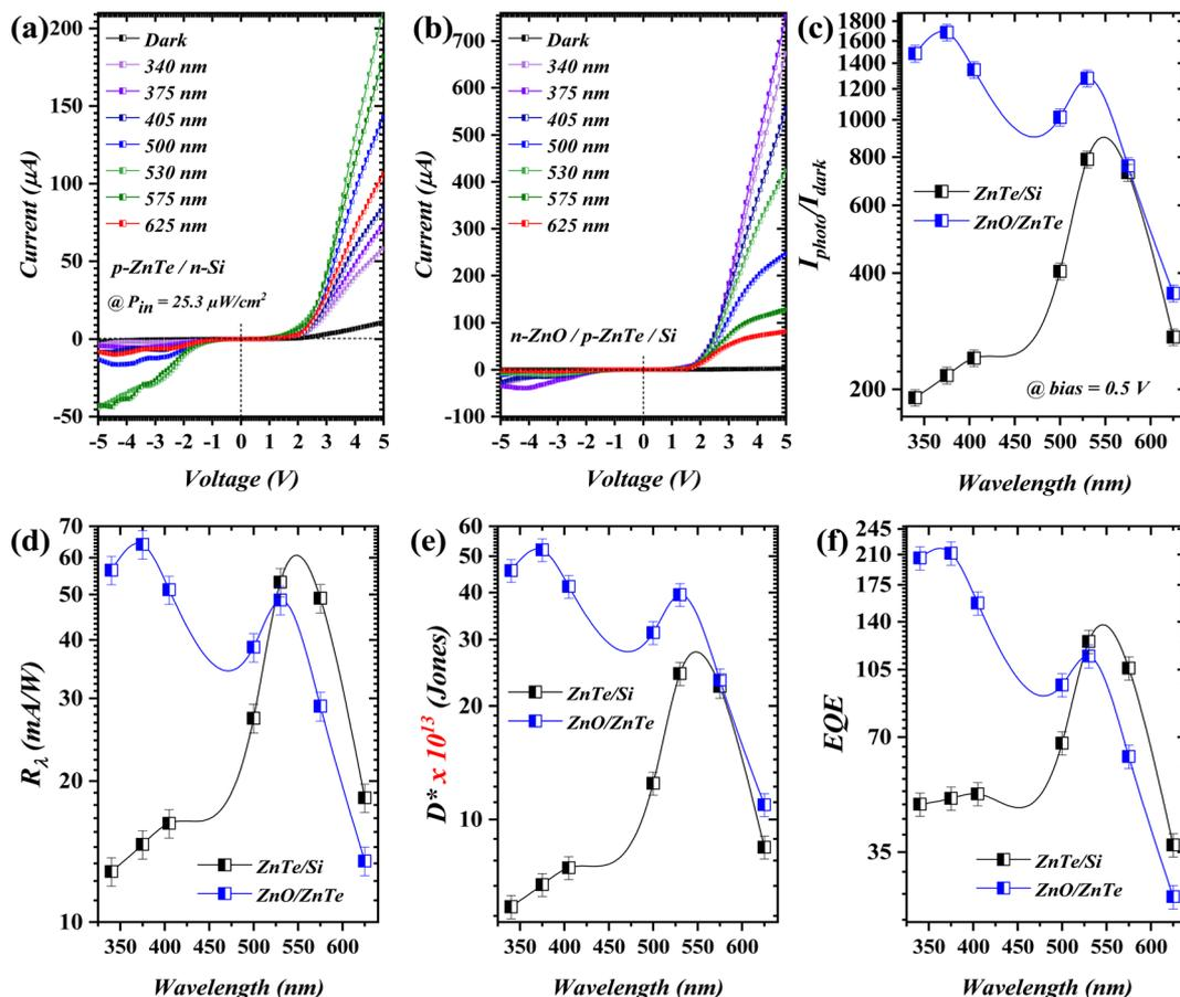
Fig. 3 Incident wavelength dependency of  $I$ - $V$  characteristics of (a) p-ZnTe/n-Si and (b) n-ZnO/p-ZnTe/Si, and the figure-of-merits are presented in (c)  $I_{\text{photo}}/I_{\text{dark}}$ , (d)  $R_{\lambda}$ , (e)  $D^*$ , and (f) EQE.
