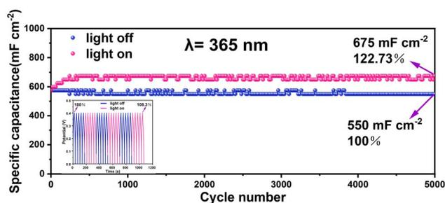
Fig. 7 Cycling performances under light off and on conditions of the CF@Cu<sub>2</sub>S-100 sample at a current density of 20 mA cm<sup>-2</sup> using a light source with a single wavelength of 365 nm.
