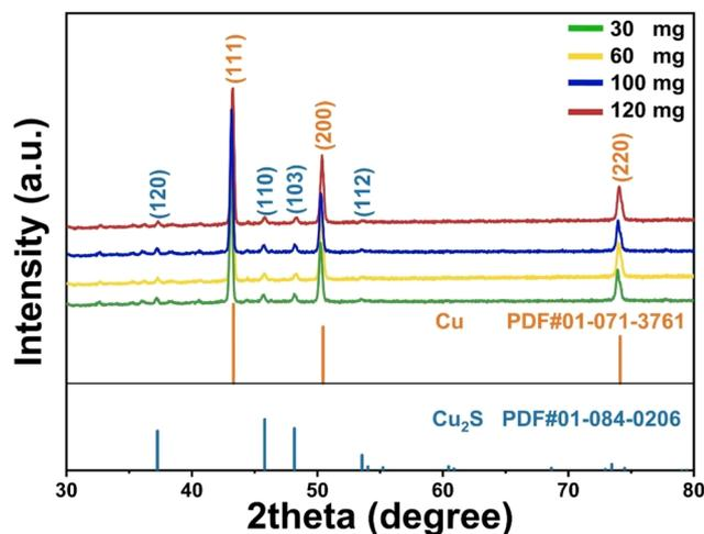
Fig. 1 XRD patterns of the CF@ $\text{Cu}_2\text{S}$  samples.
