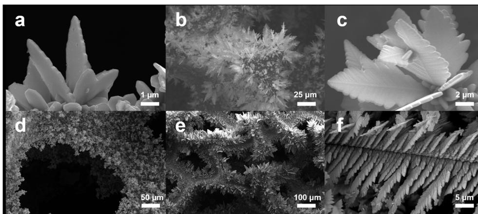
Fig. 3 SEM images of the CF@Cu<sub>2</sub>S samples: (a) CF@Cu<sub>2</sub>S-30 mg, (b) CF@Cu<sub>2</sub>S-60 mg, (c and d) CF@Cu<sub>2</sub>S-100 mg, and (e and f) CF@Cu<sub>2</sub>S-120 mg.
