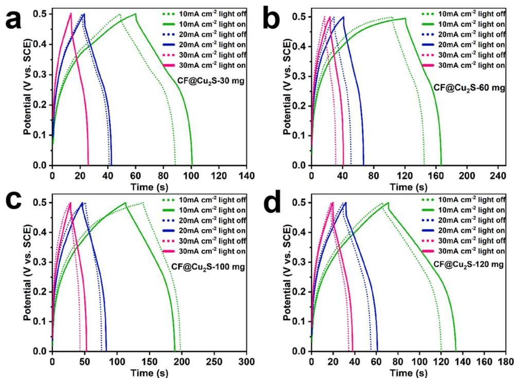
Fig. 6 GCD curves obtained at different current densities under dark and light conditions for all the samples: (a) CF@Cu<sub>2</sub>S-30 mg, (b) CF@Cu<sub>2</sub>S-60 mg, (c) CF@Cu<sub>2</sub>S-100 mg, and (d) CF@Cu<sub>2</sub>S-120 mg.
