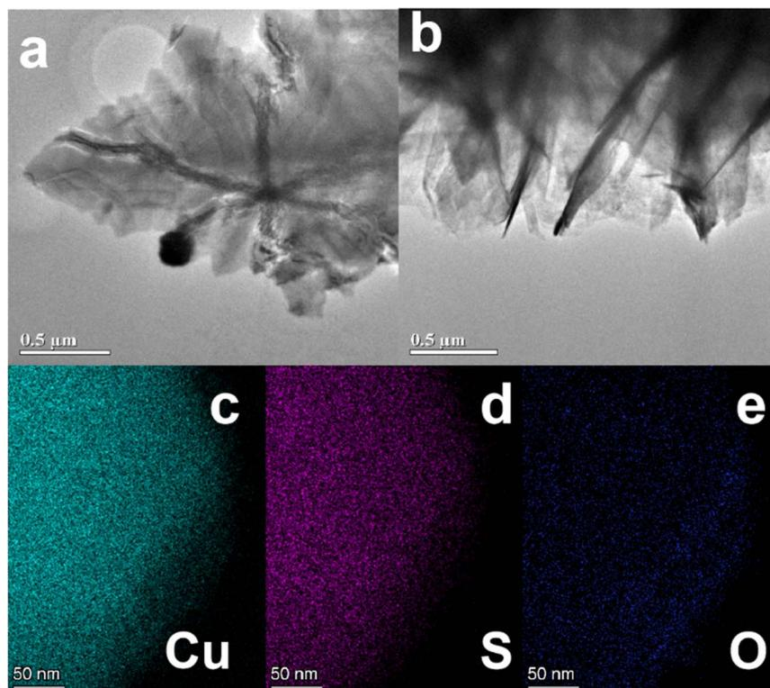
Fig. 4 (a and b) TEM images of CF@Cu<sub>2</sub>S-100 sample and (c–e) elemental mappings of Cu, S and O of the sample.
