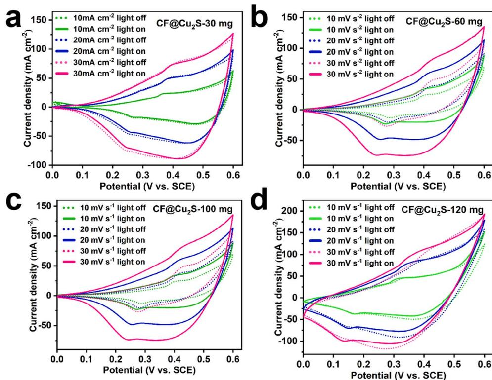
Fig. 5 CV curves obtained at different scan rates under dark and light conditions for all the samples: (a) CF@Cu<sub>2</sub>S-30 mg, (b) CF@Cu<sub>2</sub>S-60 mg, (c) CF@Cu<sub>2</sub>S-100 mg, and (d) CF@Cu<sub>2</sub>S-120 mg.
