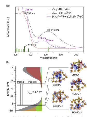
Fig. 3 (a) UV-vis absorption spectrum of the  $Au_{10}(SH)_8$  nanocluster, with oscillator strengths (f) indicated by green vertical lines. (b) Kohn–Sham energy diagram of  $Au_{10}(SH)_8$ , highlighting two dominant transitions (vertical arrows). The density of states (DOS) is color-coded to represent contributions from different atomic orbitals: total DOS (grey), Au(6s + 6p) (red), Au(5d) (orange), S(3p) (green), and H (cyan).
