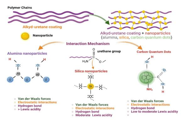
Fig. 4 Schematic representation for the interactions between alkyd-urethane resin and alumina, CQDs, or silica nanoparticles
