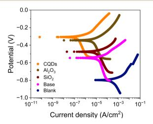
Fig. 5 Polarization curves of the uncoated coupon (blank) and alkydurethane coating (base) with 100 mg L<sup>-1</sup> of the nanoparticles evaluated in the brine saturated with CO<sub>2</sub>. The tests were carried out in a 3electrode setup with reference (Ag/AgCl) and graphite as counter electrodes at 25 °C and atmospheric pressure.
