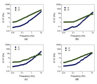
Fig. 8 Frequency dependence of alkyd-urethane viscoelastic behavior. Storage modulus (G') and loss modulus (G'') as a function of frequency for (a) alkyd-urethane resin and with loads of 100 mg L $^{-1}$  of (b) alumina (c) CQDs and (d) silica nanoparticles. The tests were carried out at 25 °C, atmospheric pressure, and dynamic rheology conditions. The linear viscoelastic region (LVR) was determined previously to the frequency sweep.
