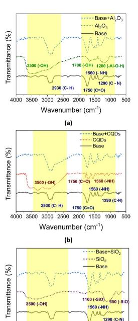
Fig. 10 Evaluation of surface interactions to the alkyd-urethane coating and nanoparticles by FTIR: (a) alumina, (b) CQDs, and (c) silica nanoparticles.
