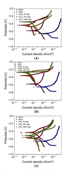
Fig. 1 Polarization curves of the blank (uncoated coupon), the base coating, and the coating with 10, 100 and 1000 mg L $^{-1}$  of (a) alumina, (b) CQDs, and (c) silica nanoparticles. The tests were carried out in a 3-electrode setup with reference (Ag/AgCl) and graphite as counter electrode at 25 °C and atmospheric pressure.
