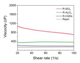
Fig. 7 Effect of alumina, CQDs, and silica nanoparticles at  $100 \text{ mg L}^{-1}$ on the alkyd-urethane resin viscosity at 25 °C and atmospheric pressure. The test was performed at steady rheology conditions.
