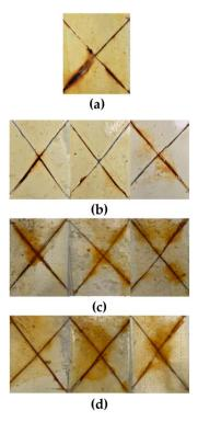
Fig. 6 Images of the corrosion resistance test for coatings of (a) alkydurethane coating (base), (b) alumina, (c) CQDs, and (d) silica nanoparticles at concentrations of  $10\,100$  and 1000 mg  $L^{-1}$ , respectively.
