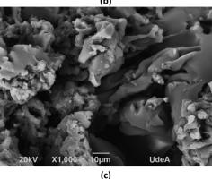
Fig. 9 Micrographs of coatings obtained by SEM: (a) alkyd-urethane coating, (b) coating with 100 mg  $L^{-1}$  of alumina nanoparticles, and (c) coating with 100 mg  $L^{-1}$  of CQDs.
